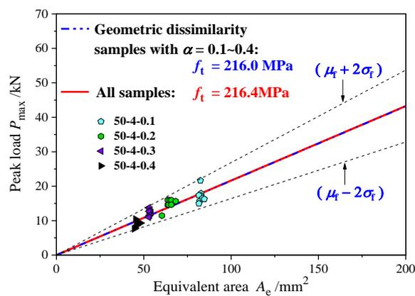
Fig. 6 Tensile strength of geometrical dissimilar samples with different  $\alpha$ -ratios
