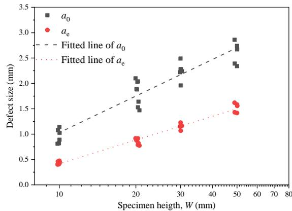
Fig. 8 Semi-logarithmic fitting between material defect size with sample height
