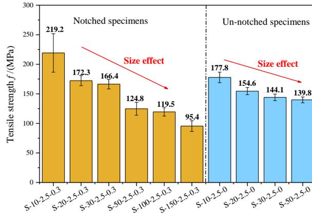
Fig. 1 Size effect phenomenon in brittle tensile strength under bending load
