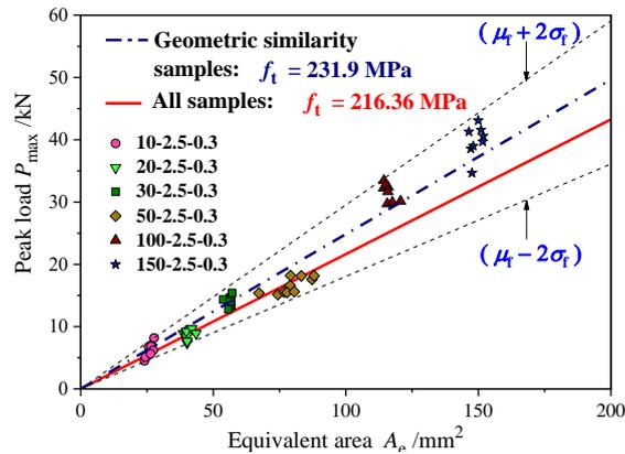
Fig. 5 Tensile strength of geometrical similar samples with different heights
