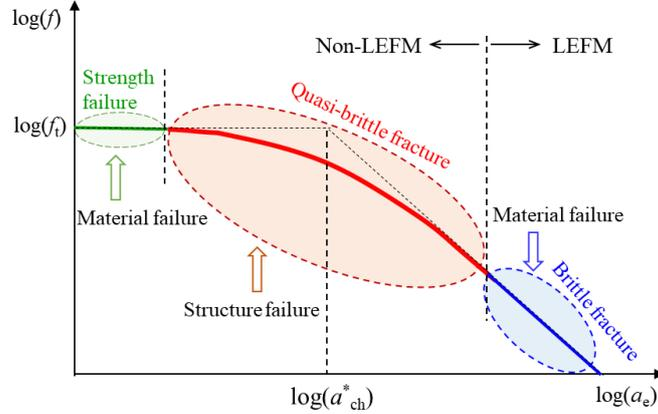
Fig. 3 Size effect analysis of PSBL by equivalent crack  $a_e$
