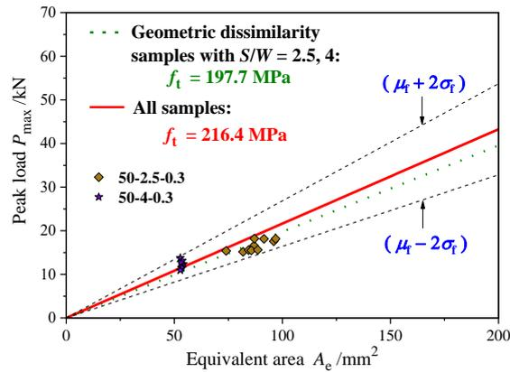
Fig.7 Tensile strength of geometrical dissimilar samples with S/W as 2.5 and 4
