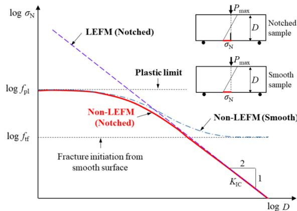
Fig. 2 Schematic diagram regarding the size dependency in a double-logarithmic scale
