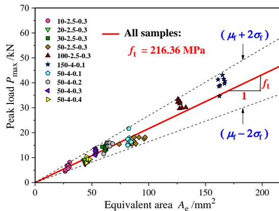
**Fig. 4** Linear  $P_{max} - A_e$  relation fitting of all notched samples
