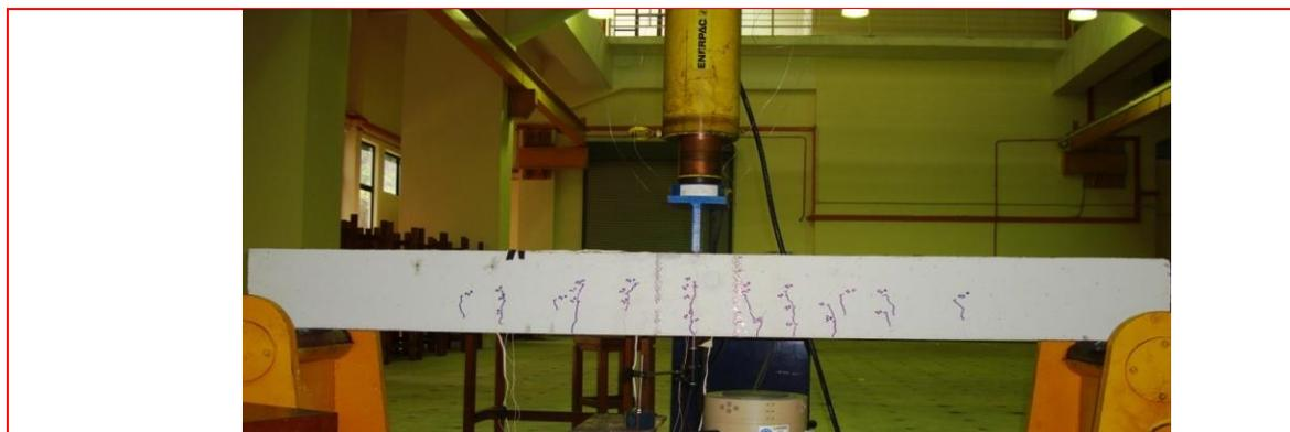
Fig. 4 Beam under static test – flexural scenario
