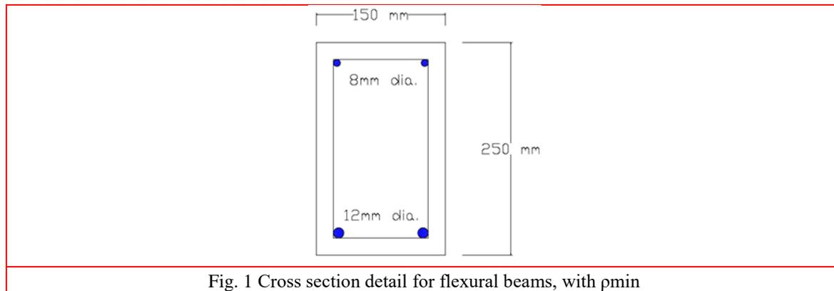
Fig. 1 Cross section detail for flexural beams, with  $\rho_{min}$
