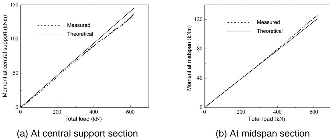
Fig. 6 Load-flexural moment curves of specimen G-1
