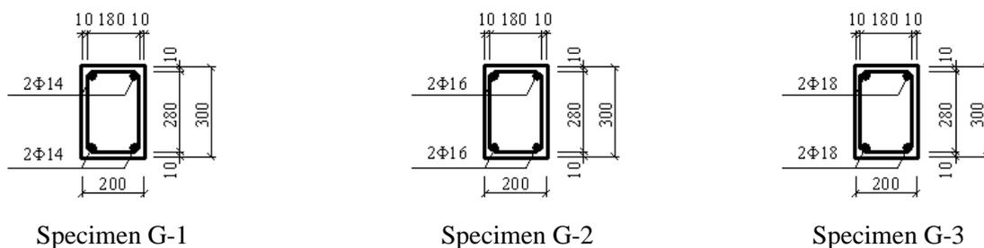
Fig. 1 Sections and reinforcement detail of specimens (dimensions in mm)
