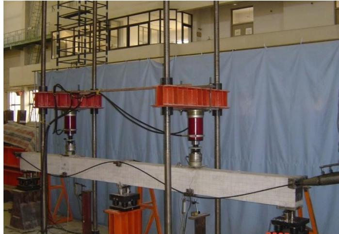
Fig. 3 Loading test of specimens
