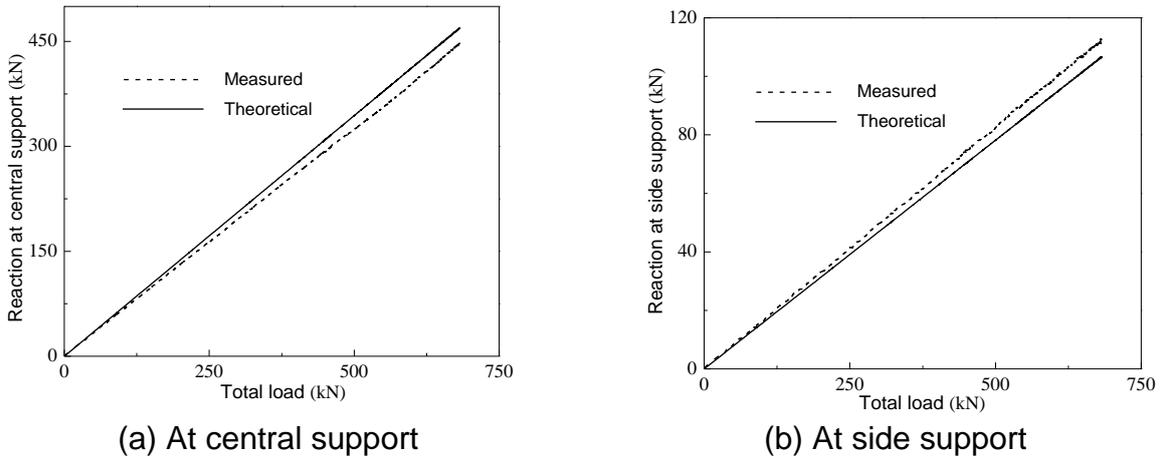
Fig. 5 Load-support reaction curves of specimen G-3
