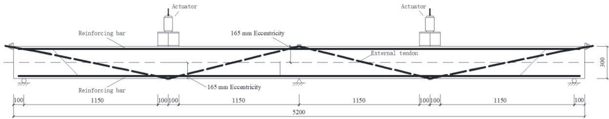
Fig. 2 External prestress tendon profile of specimens (dimensions in mm)
