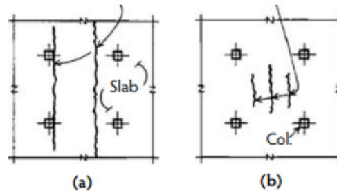
**Fig.1.** Reflected ceiling view of slabs illustrating crack formation in (a) post-tensioned slab; (b) reinforced concrete slab. (Nawy, 2008)
