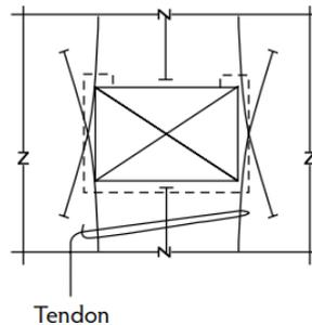
**Fig.2.** Arrangement of tendons as to prevent the formation of cracks around an opening. (Nawy, 2008)
