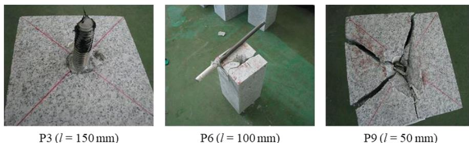
Fig. 1 Condition of specimens with 16 mm diameter bar at the end of the loading
