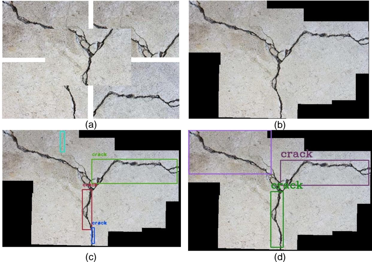
**Fig. 1** The process of structural damage detection
