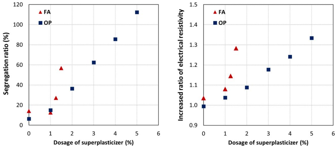
Fig. 5 (a) Increased ratio of electrical resistivity by dosage of superplasticizer
