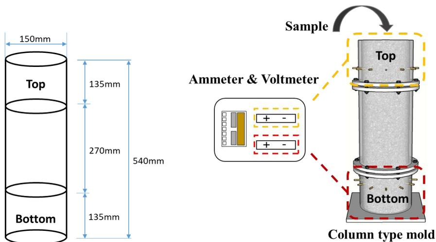
Fig. 2 Electrical resistivity measurement mold for evaluation of concrete segregation
