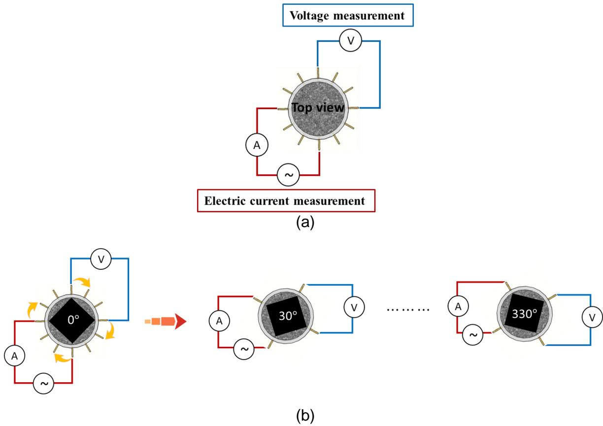
Fig. 3 (a) Electrical resistivity measurement system using electrode square configuration
