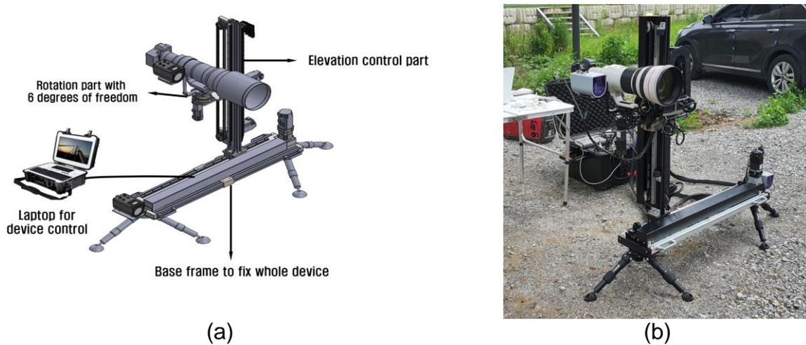
Fig. 2. Automated Image Capturing Device: (a) Concept Drawing and (b) Image of the device in use.
