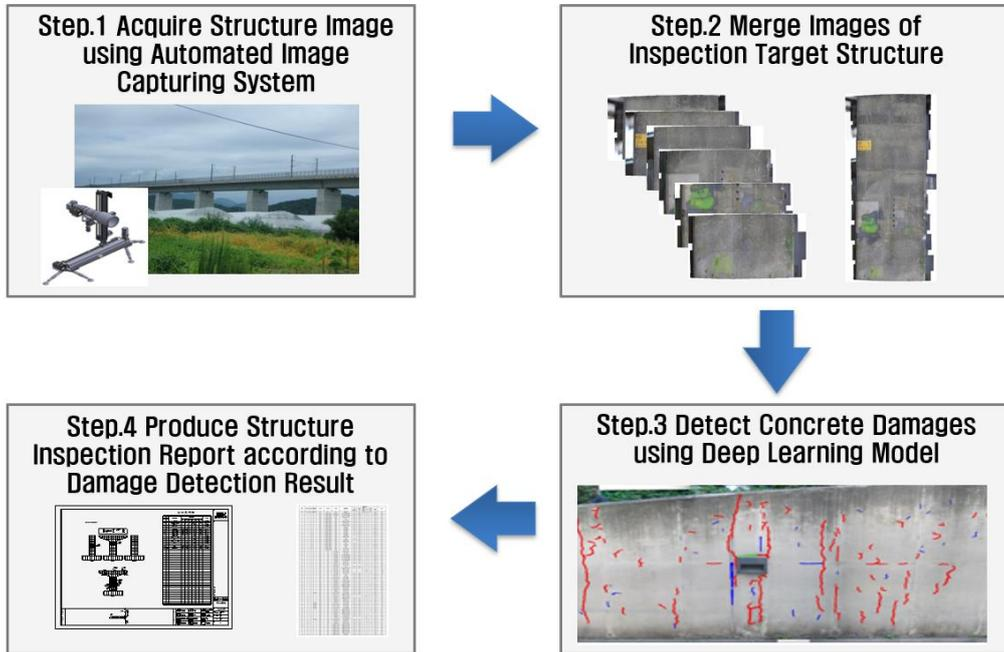
Fig. 1. Overall Concrete Damage Detection Framework using an Automated Image Capturing Device and Deep Learning Model.
