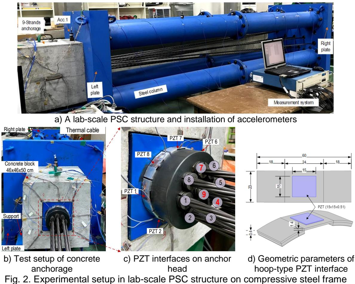
Fig. 2. Experimental setup in lab-scale PSC structure on compressive steel frame
