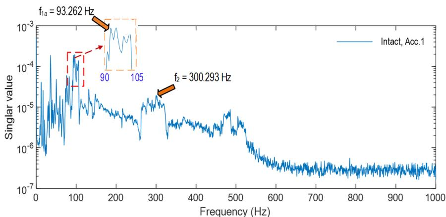
Fig. 4 Frequency response function using acceleration signals of Acc.1 in Case 1
