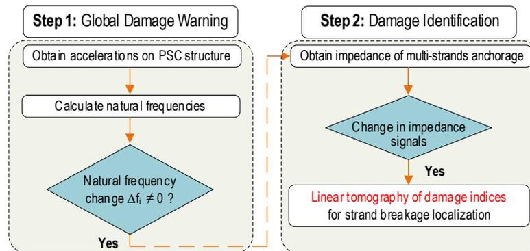
Fig. 1. Hybrid health monitoring scheme for PSC structure
