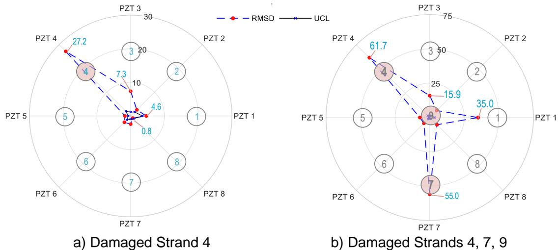
Fig. 6 Linear tomography of RMSD indices (%) under damaged Strand 4 and damaged Strands 4, 7, 9 in frequency range 5-35 kHz
