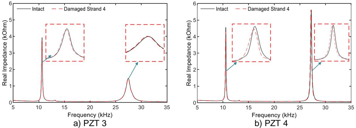
Fig. 5 Impedance responses of PZT sensor under breakage of Strand 4
