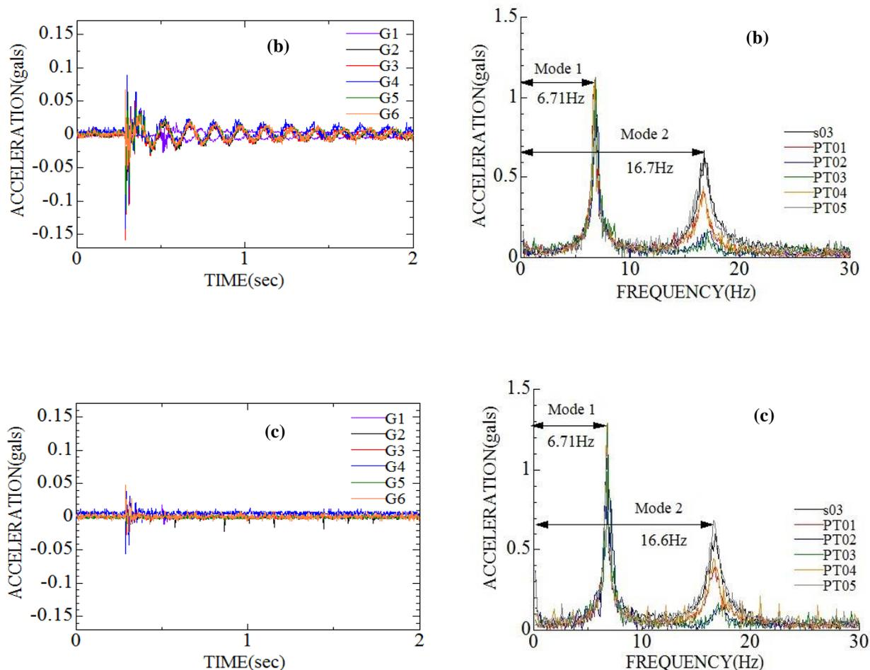
**Fig. 6** Measured acceleration and frequency responses of the bridge (a) time-history and natural frequency result of load dropped on the center of the bridge (b) time-history and natural frequency result of load dropped on G2 (c) time-history and natural frequency result of load dropped on G5.
