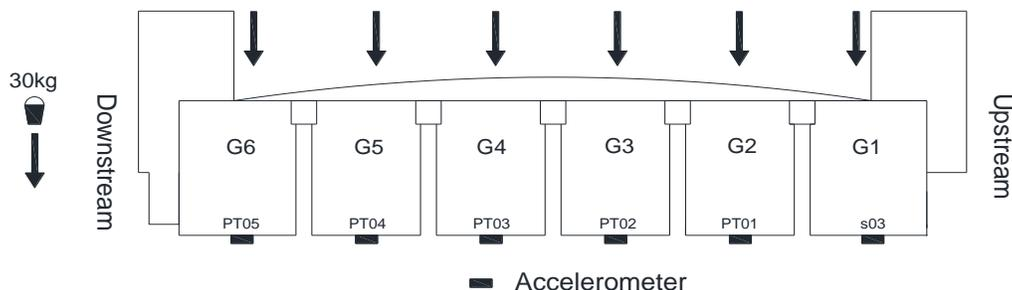
**Fig. 4** Layout of data acquisition system using accelerometers
