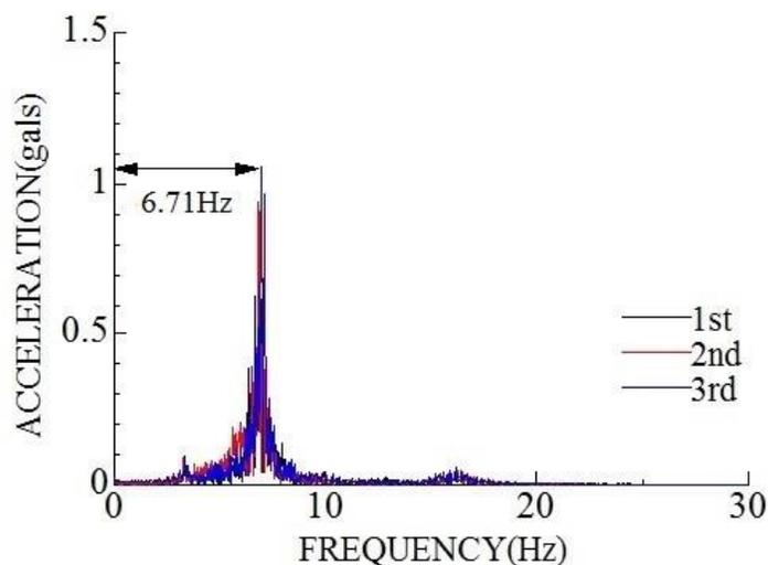
**Fig. 8** Vibration response acquired from G1 girder
