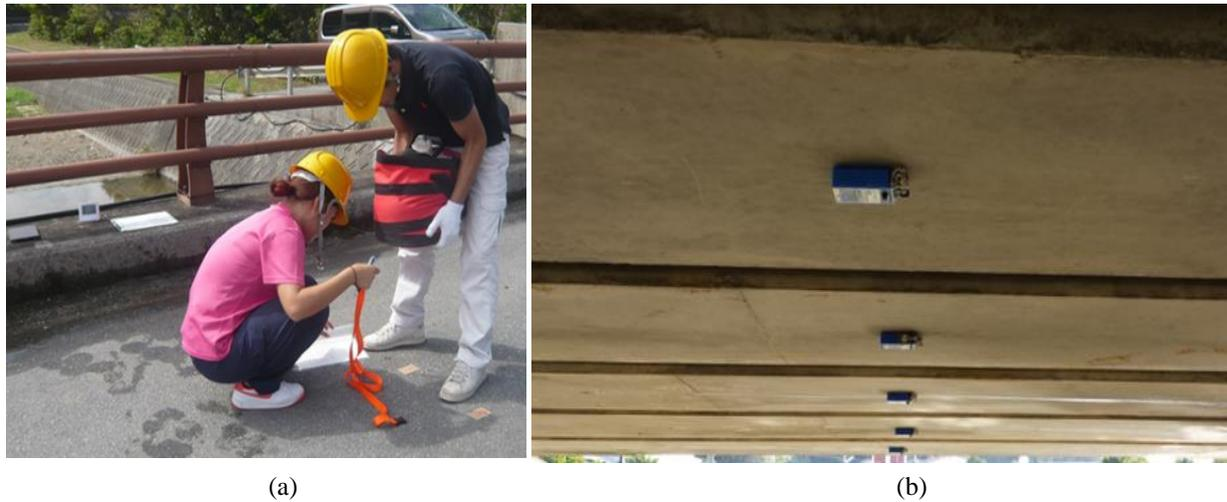
**Fig. 5** (a) dropping load illustration (b) positions of accelerometers on the bridge's girders
