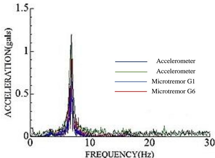
**Fig. 12** Comparison of the accelerometers' and microtremors' results
