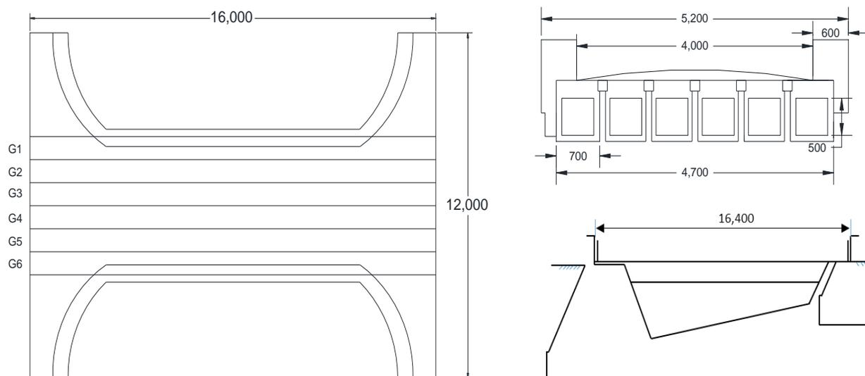
**Fig. 2** Top, cross-sectional and transversal views of the bridge
