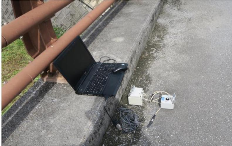
**Fig. 7** Data acquisition from microtremor sensors
