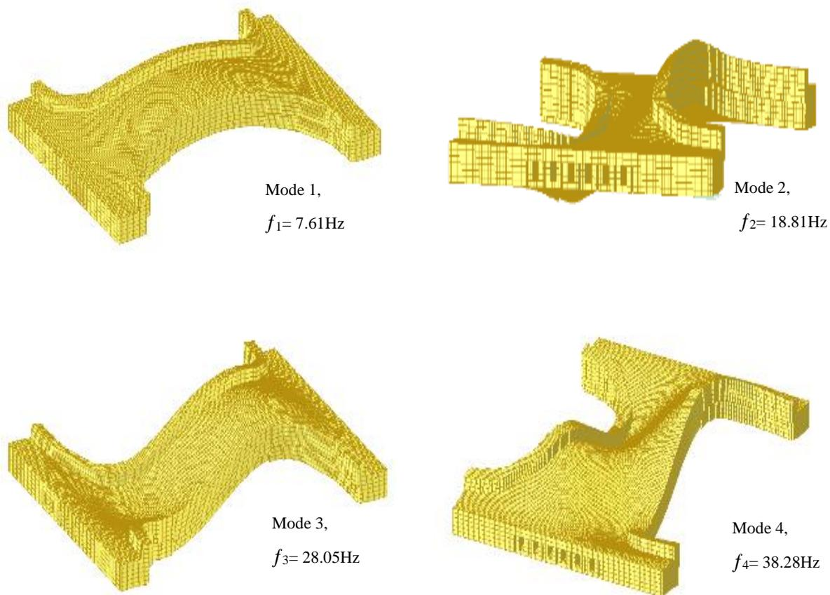
**Fig. 11** Plotted mode shapes and their corresponding natural frequency of eigenvalue analysis of the bridge
