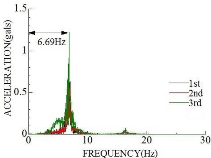
**Fig. 9** Vibration response obtained from G6 girder
