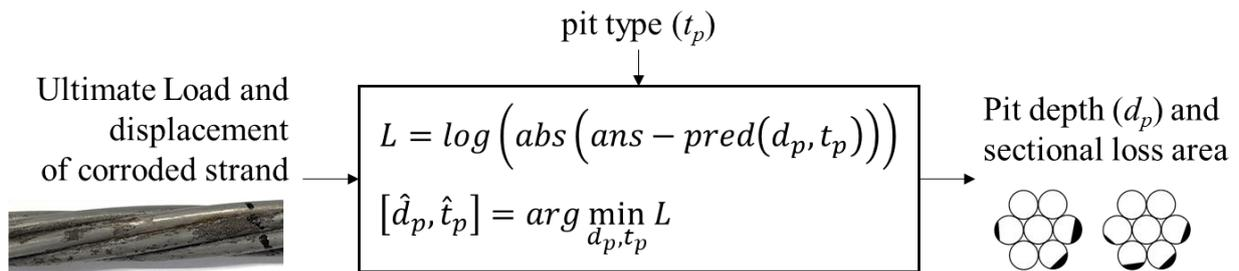
Fig. 3. Inference method to evaluate the corrosion configurations.
