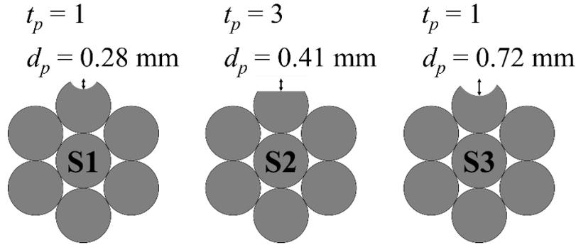
Fig. 2. Test specimens of corroded strands.
