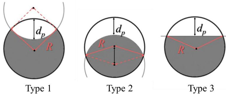
Fig. 1. Pit shapes for FE analysis (Jeon *et al.* 2019).
