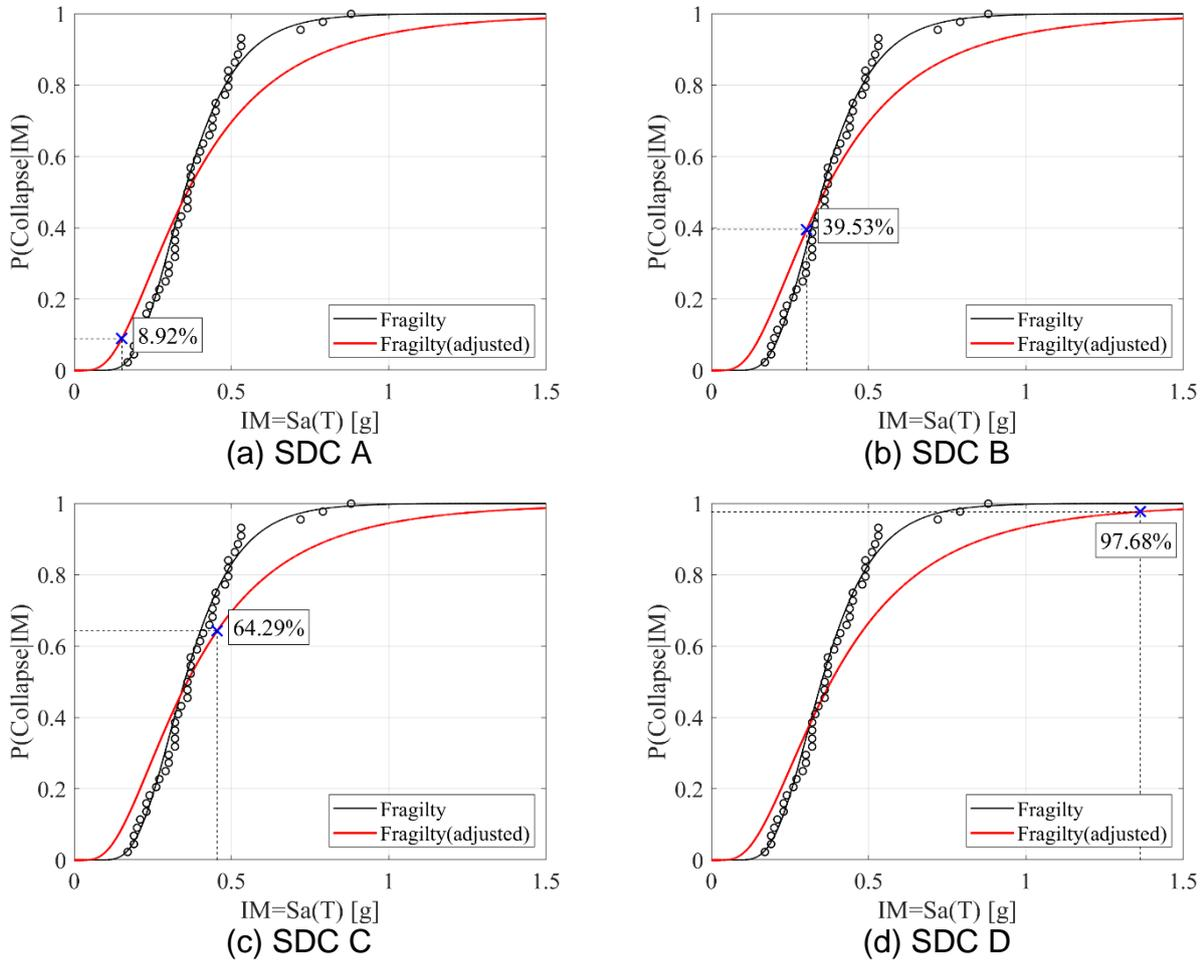
Fig. 5 Adjusted collapse fragility curve according to SDC
