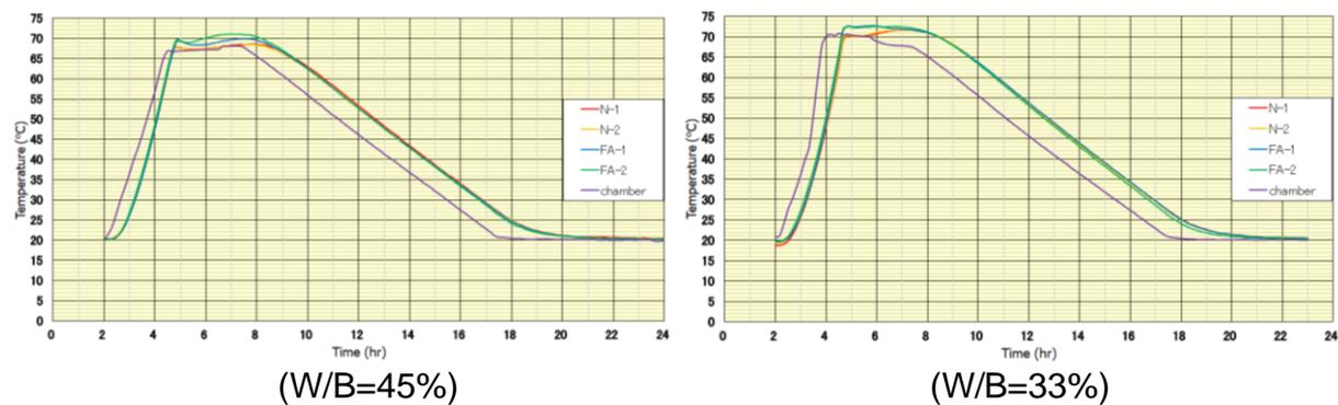
Fig.1: Temperature History of Steam Curing
