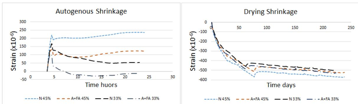
Fig.3: Autogenous Shrinkage and Drying Shrinkage
