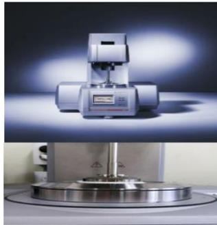
Fig. 1 Rheometer used for cement paste rheology measurements
