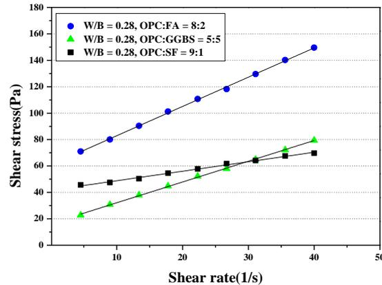
Fig. 3 Results of measuring the rheological properties of mixtures with different binders (Binary system)
