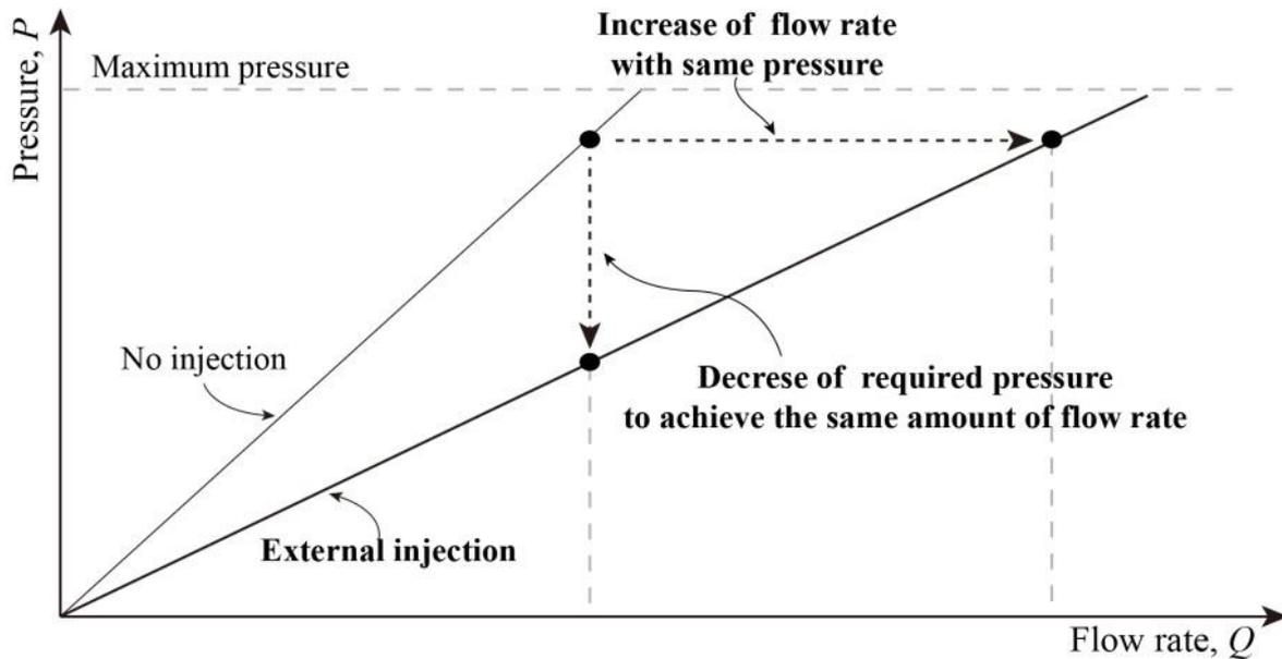
Fig. 2 Improvement of pumpability by injecting viscosity
