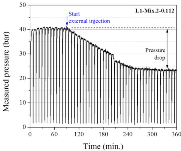
Fig. 9 Measured pressure during pumping
