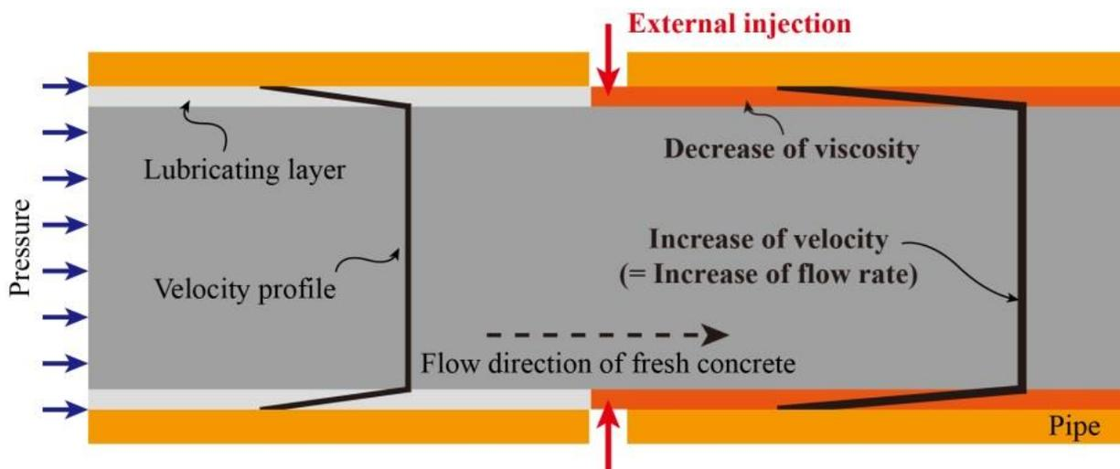
Fig. 1 Mechanism of external injection method
