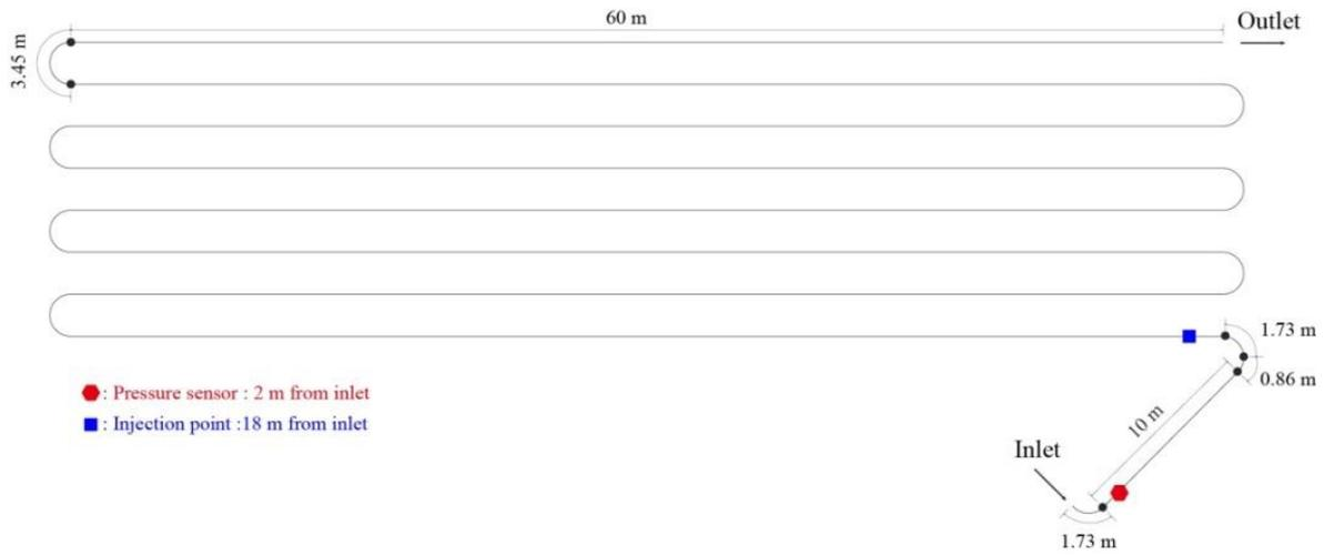
Fig. 8 Detail of 514 m pipeline(L3)
