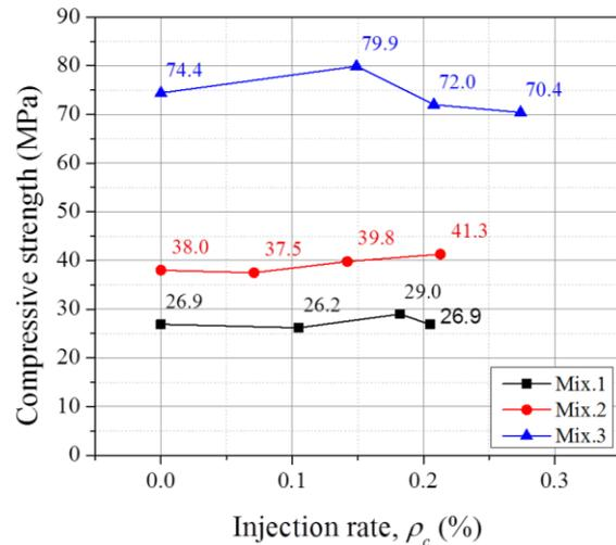
Fig. 12 Variation of compressive strength according to injection rate
