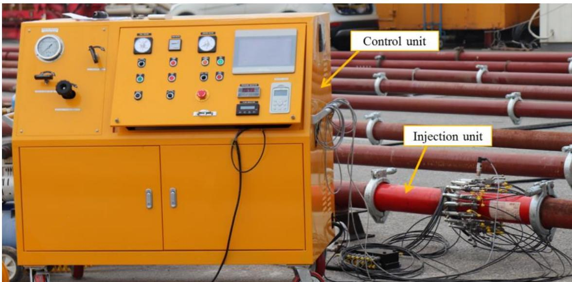
Fig.3 Installation of injection device in the pumping circuit
