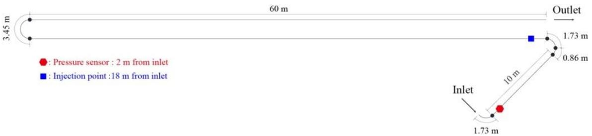
Fig. 7 Detail of 137 m pipeline(L1)
