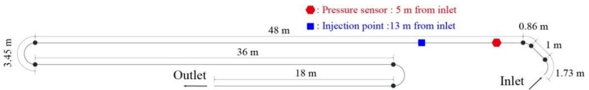
Fig. 5 Detail of 112 m pipeline(L1)
