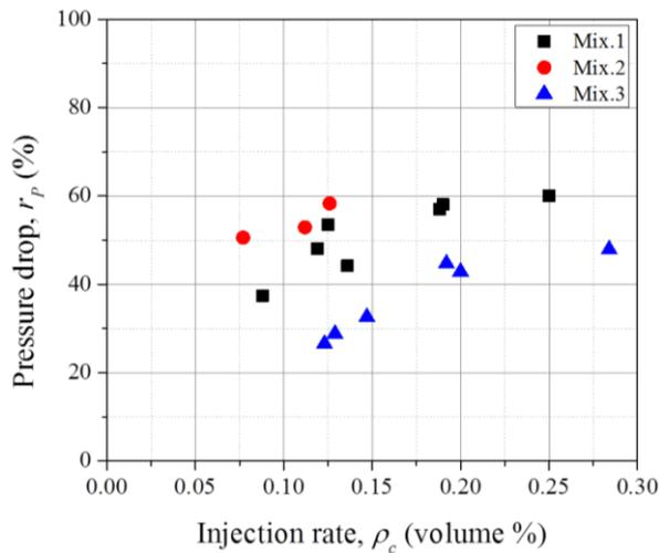
Fig. 11 Relationship between injection rate( $\rho_c$ ) and pressure drop( $r_p$ )
