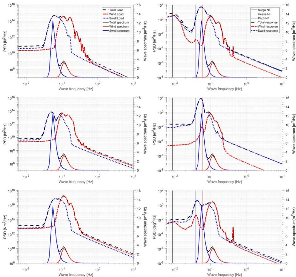
Fig. 5 Load and global response PSD (surge, heave, pitch); (black dot : Total load & response, red dot : wind sea load & response, blue dot: Swell load & response, black line : Total wave spectrum, red line: wind sea wave spectrum, blue line: Swell wave spectrum)
