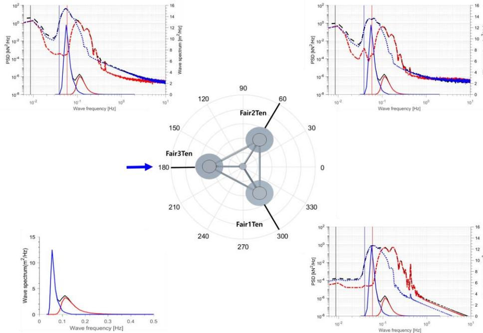
Fig. 6 Power spectrum density of tensions in the mooring lines(black dot : Total FairTen, red dot : wind sea FairTen, blue dot: Swell FairTen, black line : Total wave spectrum, red line: wind sea wave spectrum, blue line: Swell wave spectrum)
