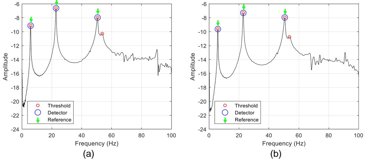
**Fig. 2** Peak identification performance comparison of peak detector and threshold-based approaches
