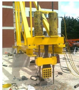
Fig. 7 Loading system: (a) triangular steel truss; (b) hydraulic jacks and dovetail shaped steel plate
