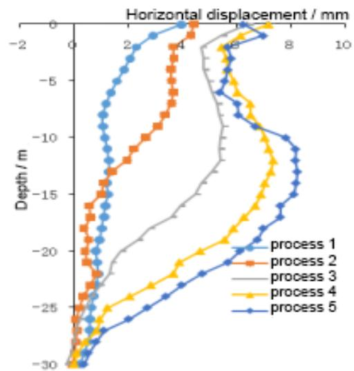
Fig. 4 Horizontal deformation of ZQT7 pile Fig. 5 Horizontal deformation of ZQT9 pile
