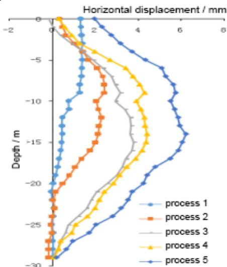
Fig. 2 Horizontal deformation of ZQT3 pile
