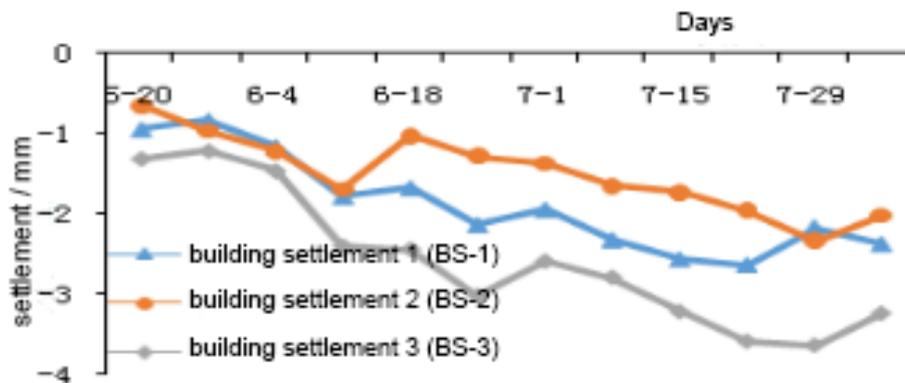
Fig. 9 Building settlement monitoring deformation curve
