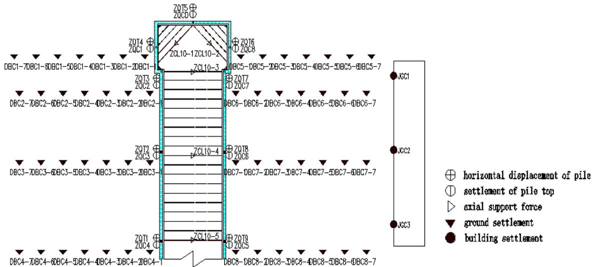
Fig. 1 Subway line 10 excavation layout plan
