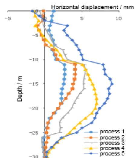
Fig. 3 Horizontal deformation of ZQT5 pile
