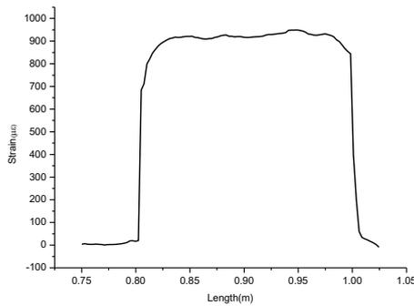
(a) Strain distribution with 0.5mm adhesive layer thickness
