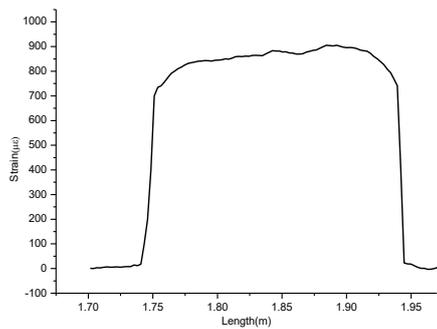
(c) Strain distribution with 2.5mm adhesive layer thickness
