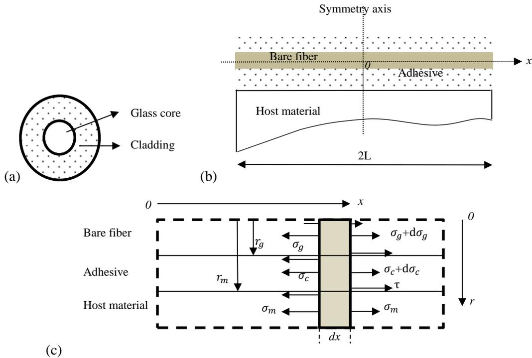
**Fig.1** Coordinate system and free body diagram of longitudinal section of optical fiber;
