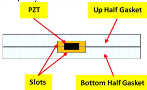
Fig. 3 The design of smart washer
