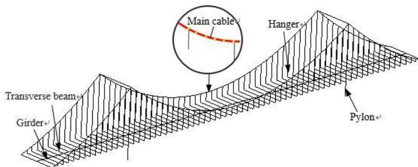
**Fig. 9** FE model of the bridge
