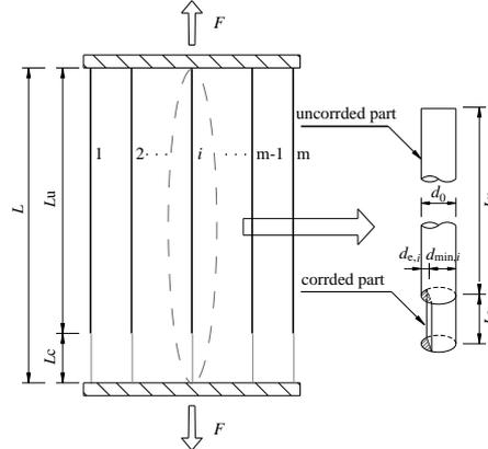
Fig. 5 Modified model of a hanger
