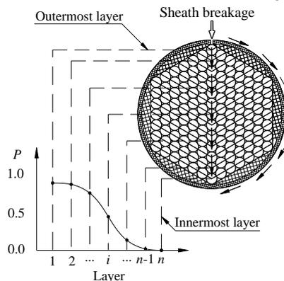
Fig. 4 Corrosion distribution in a cross section of a hanger
