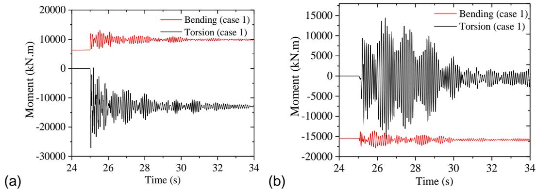
Fig. 14 Responses of the girder (a) near the broken hanger (b) near the tower
