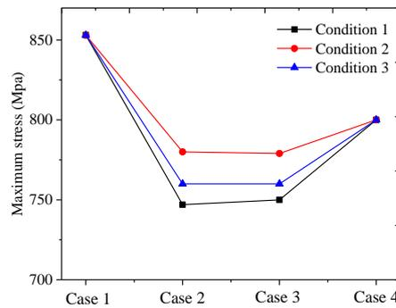
**Fig. 13** Maximum tensile stress of the hanger numbered 22
