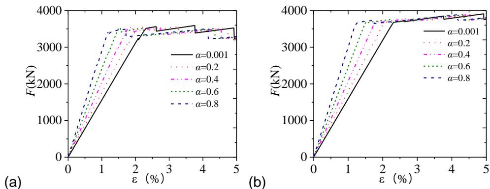
Fig. 7 Force-strain curves of the hanger when  $d_{e,1}$  is 1mm (a)  $R_e=0.9$  (b)  $R_e=0.5$
