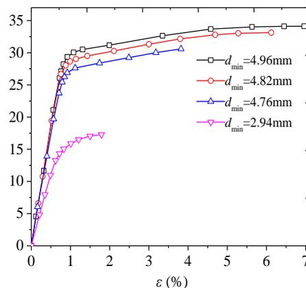
Fig. 3 Force-strain curves of one single wire
