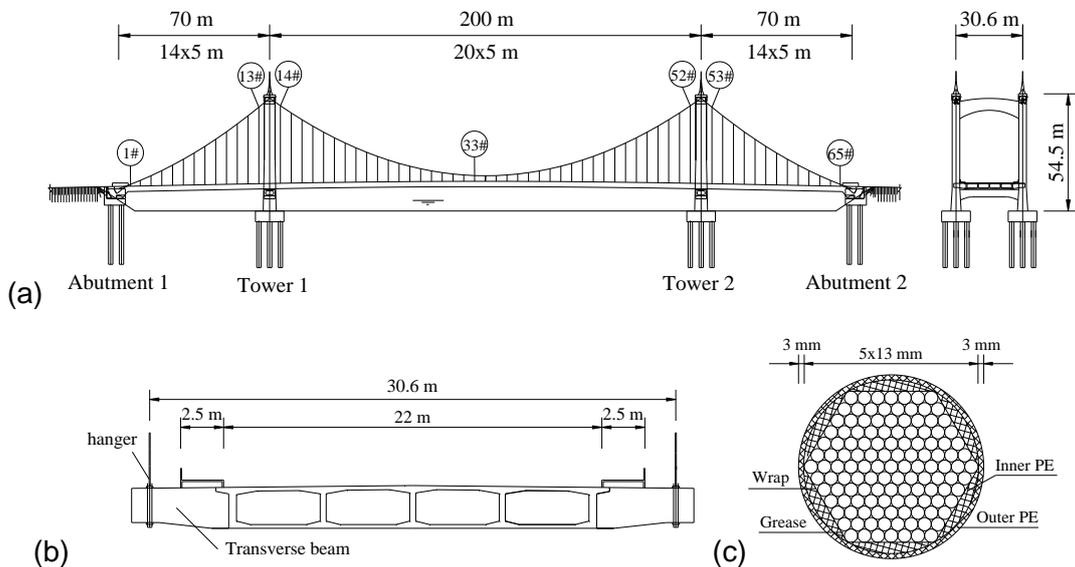
**Fig. 8** Prototype self-anchored suspension bridge (a) general layout (b) cross section of stiffening girder (c) cross section of hanger
