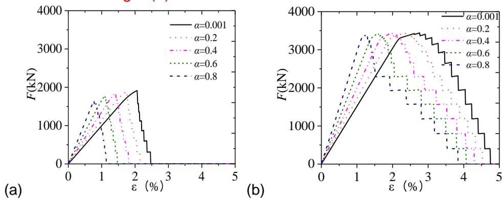
Fig. 6 Force-strain curves of the hanger when  $d_{e,1}$  is 4mm (a)  $R_e=0.9$  (c)  $R_e=0.5$
