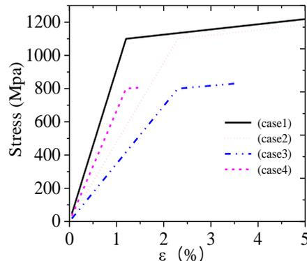
Fig. 11 Load-strain curves of the hanger
