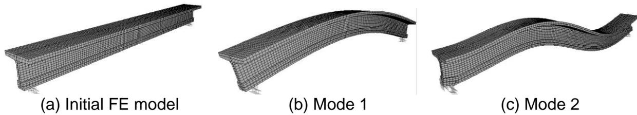
Fig. 3. FE analysis of PSC beam
