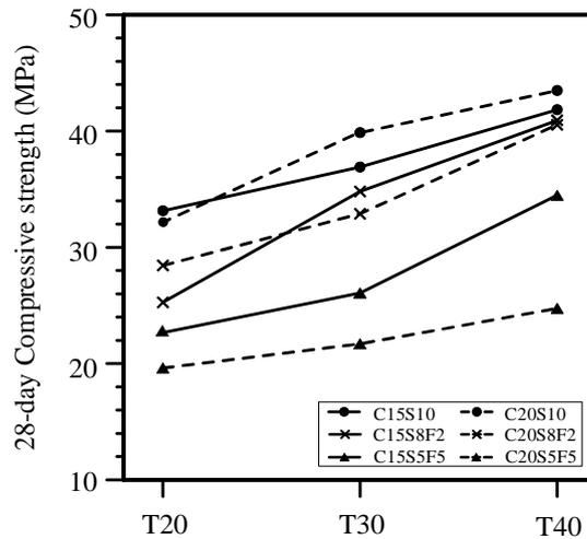
Fig. 3 The effect of additional CFBC fly ash in compressive strength
