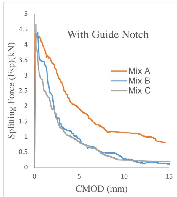
Figure 5. Splitting force vs. CMOD for with guide notch specimens
