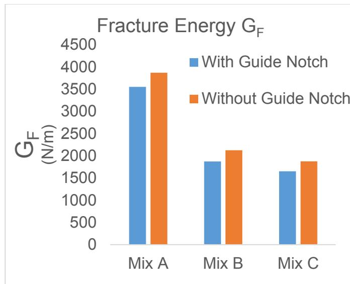
Figure 6. Fracture Energy variation for with Guide notch and without Guide notch
