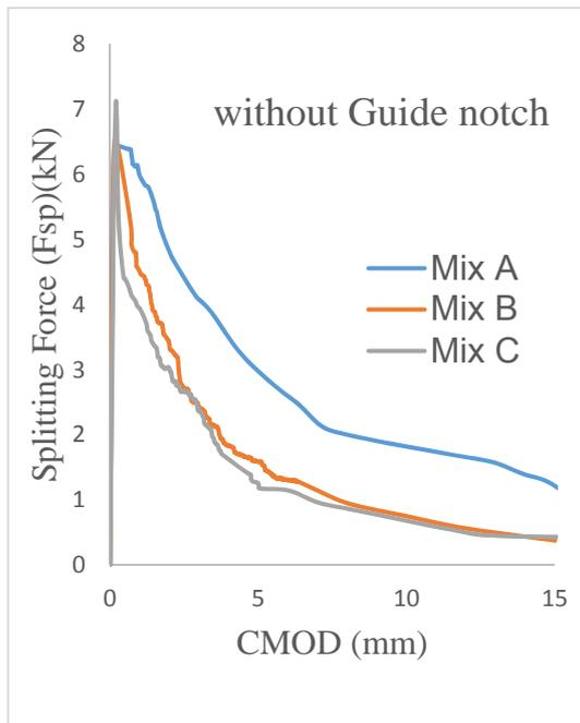
Figure 4. Splitting force vs. CMOD for without guide notch specimens
