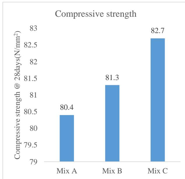
Figure 3. Compressive strength results of Fibre Reinforced Self compacting Concrete
