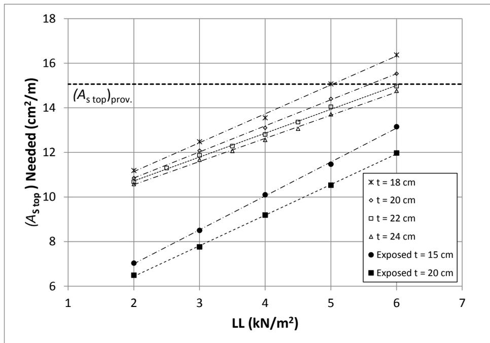
Fig. 9. Top reinforcement requirements versus surface live load for completely exposed slab panels and those covered with drain system.
