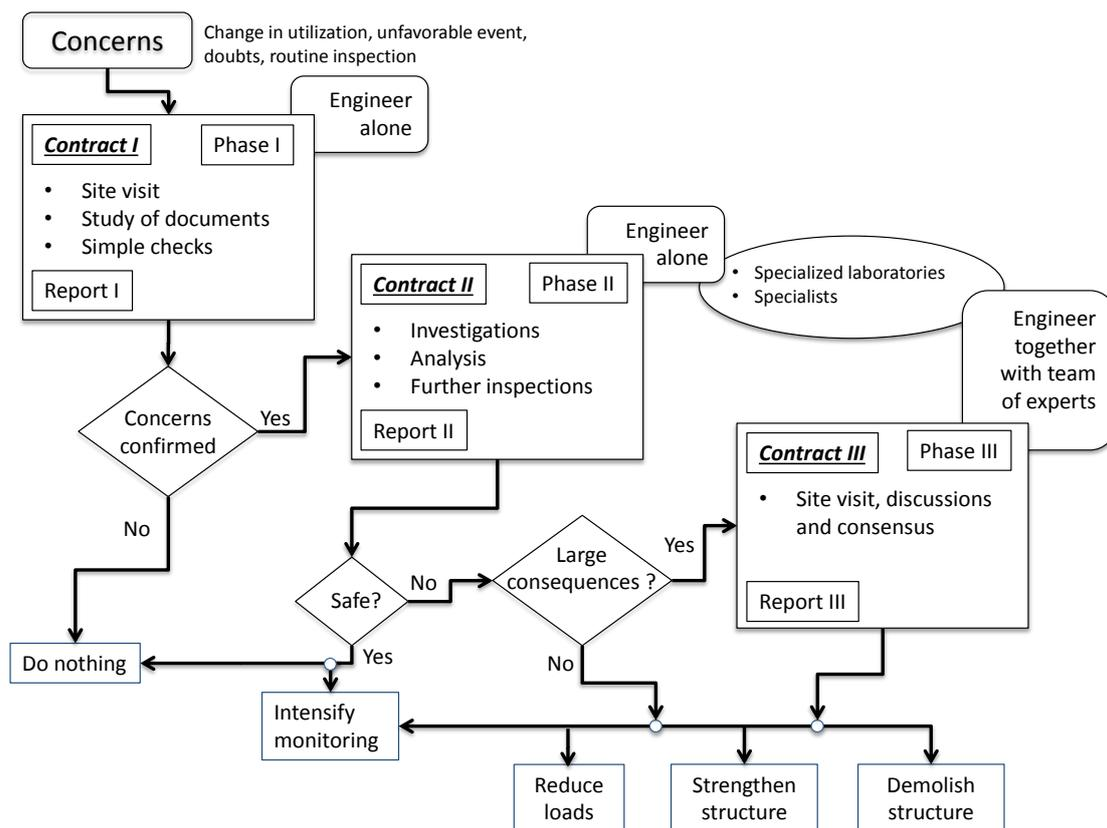
Fig. 1. Illustration of the three phases approach (RILEM 2001).
