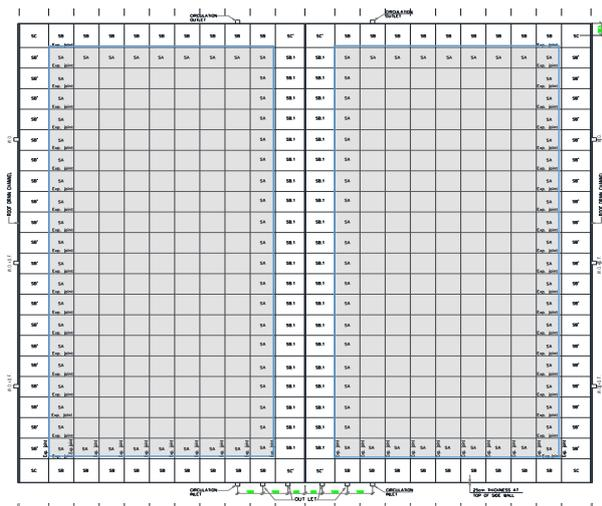
Fig. 3. Arrangement of roof slab panels of a typical 200x200 m underground water reservoir.
