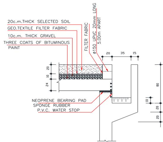
Fig. 4. Typical section through the gutter and the roof drainage system.
