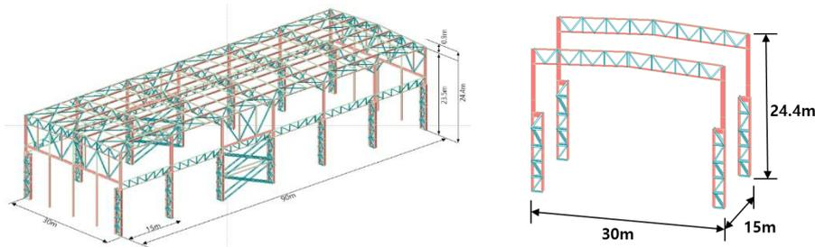
Fig. 1 Prototype of existing industrial building and its unit frame
