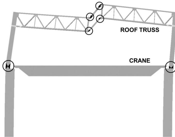
Fig. 6 Yield mechanism of proposed vierendeel-truss system
