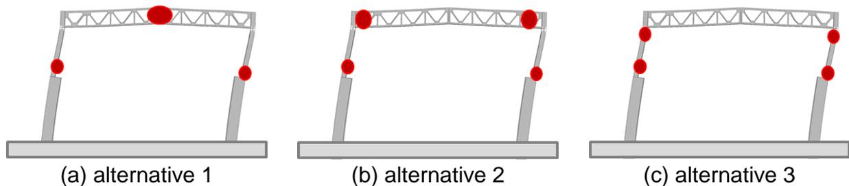
Fig. 3 Alternatives for yield mechanism
