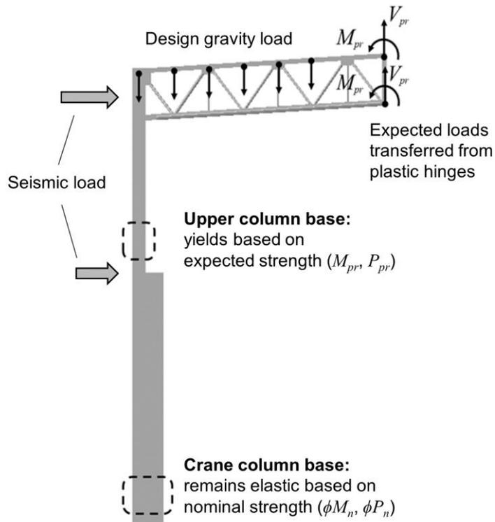
Fig. 5 Capacity design procedure illustrated
