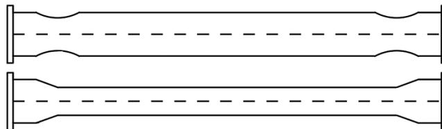
Fig. 11 Robust vierendeel beam end details: RBS (top) and flare connection (bottom)
