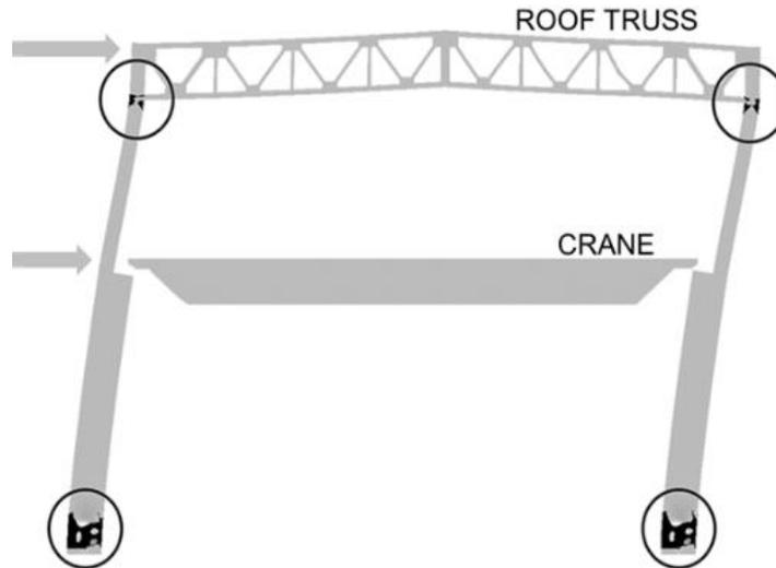
**Fig. 2** Yield mechanism from pushover analysis of the prototype (black region shows yielding)
