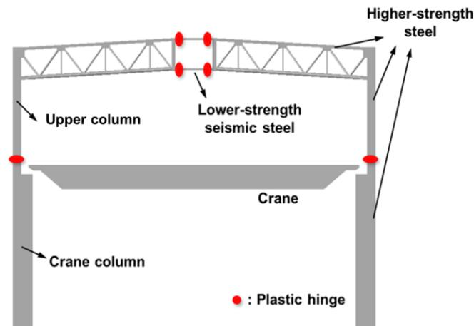
Fig. 4 Key concepts for vierendeel-truss system proposed
