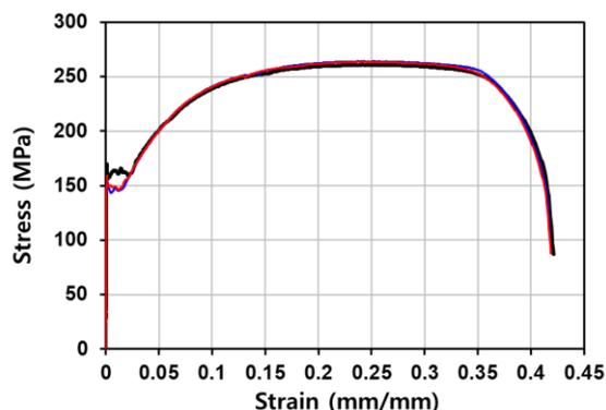
Fig. 7 Stress-strain curves from 160MPa LYP steel
