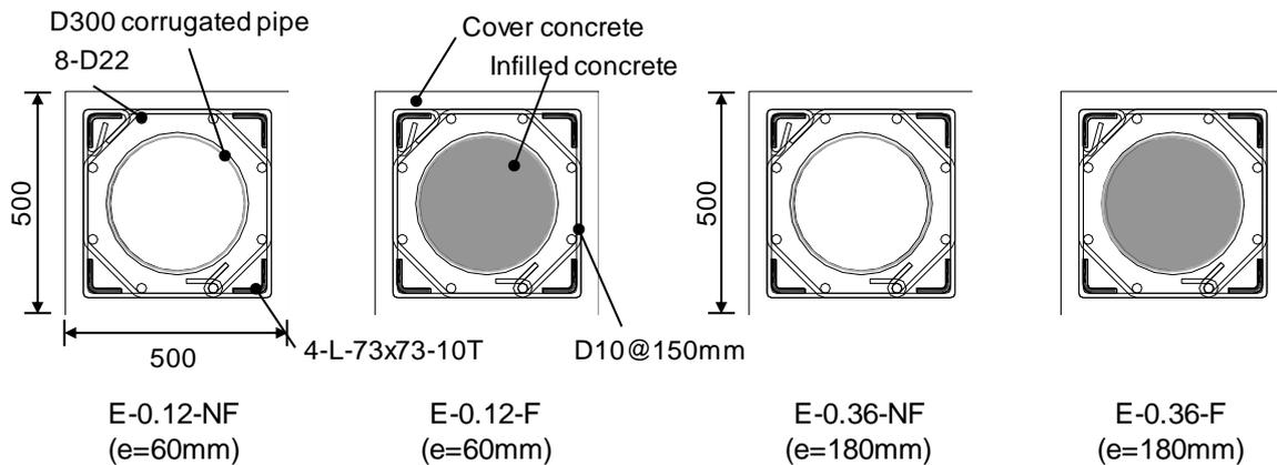
Fig. 1 Specimen section
