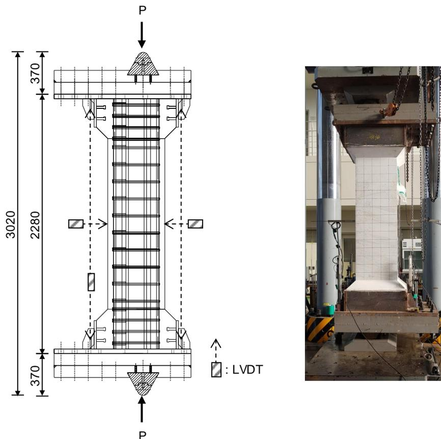
Fig. 2 Test setup of eccentric compression test
