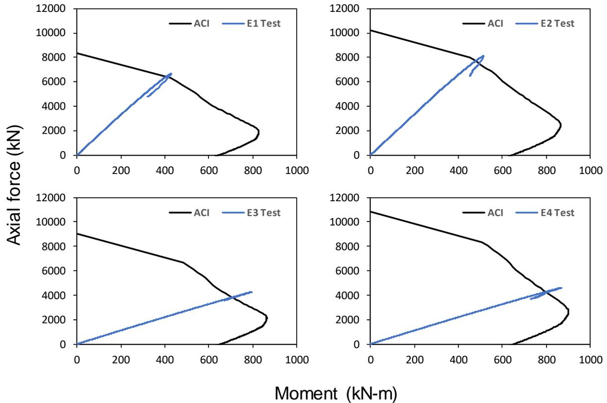
Fig. 4 Comparison test results with ACI code provision
