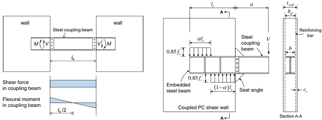
Fig. 1 Coupled PC wall-steel link beam system and its ultimate limit state
