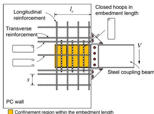
**Fig. 4** Suggested reinforcement detailing for hybrid PC wall-steel link beam systems
