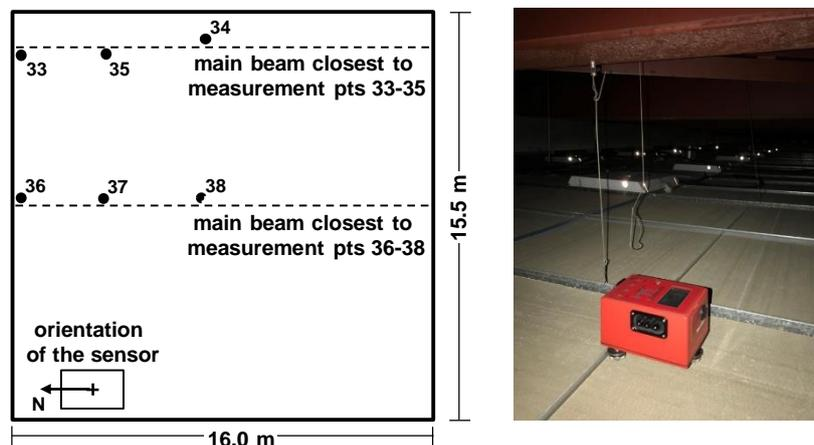
**Fig. 2** Schematic plan of the ceiling with location of the measurement points (left), and a picture of the sensor (right)
