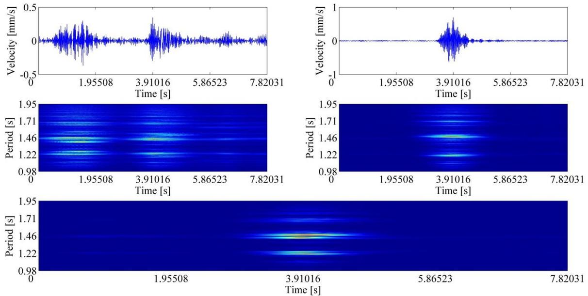
**Fig. 3** Time-frequency domain analysis (measurement points 33 and 35): velocity records (upper row), time vs pseudo-period from continuous wavelet transform (central row), time vs pseudo-period from the cross wavelet spectrum (bottom row); the plots refer to the time-window around the peak velocity
