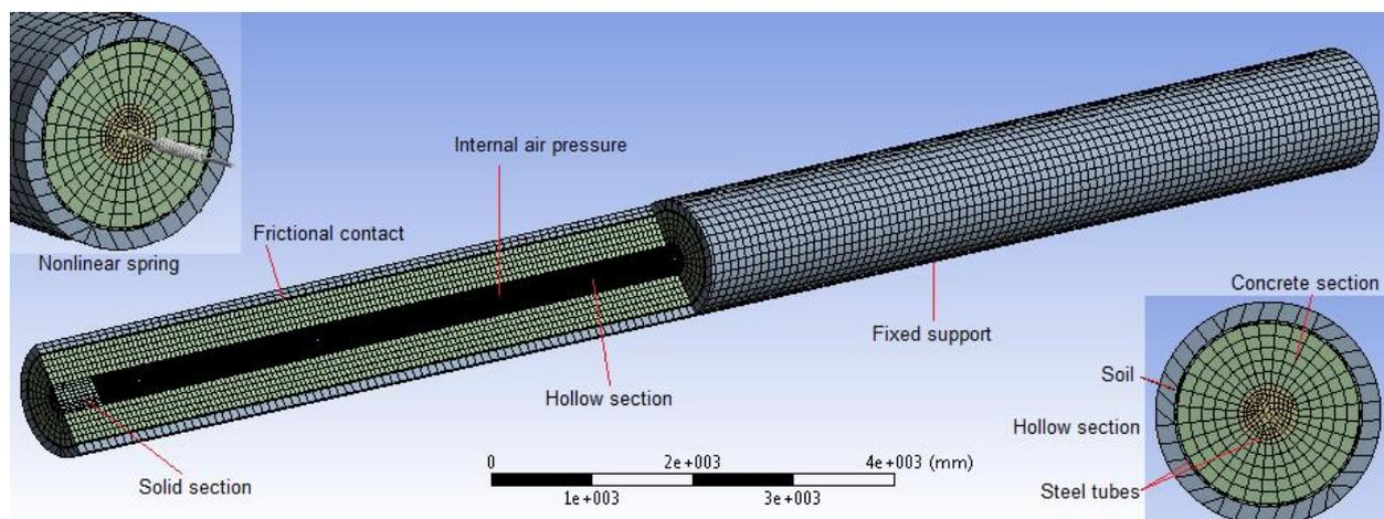
Fig. 1 3D model of the energy pile
