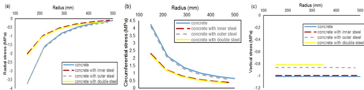
Fig. 2 Stress states of concrete along the radial direction
