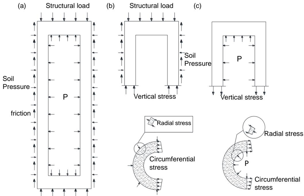
Fig. 1 Stress states under (a) applied loads, (b) structural load, (c) internal air pressure.
