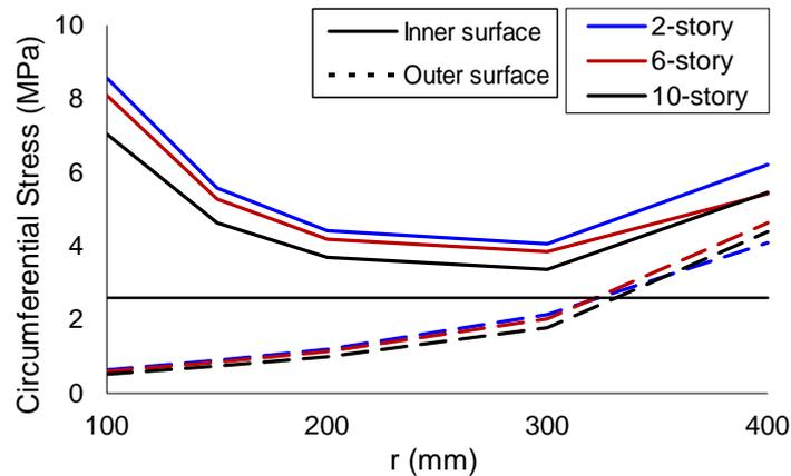
Fig 3. Stress distribution of the pile along the circumferential direction
