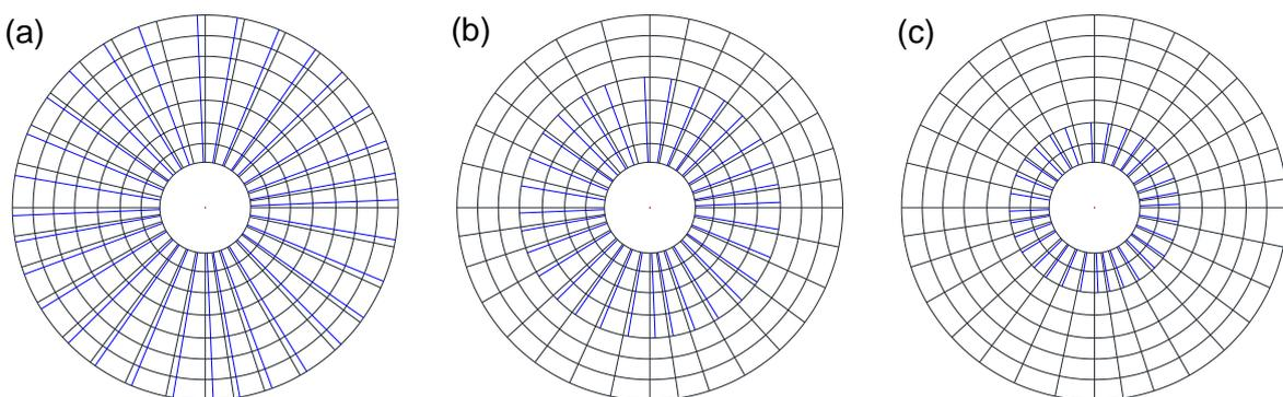
Fig. 4 Crack penetrations with hoop reinforcement ratio of (a) 2.3%, (b) 2.5% and (c) 3.1%.
