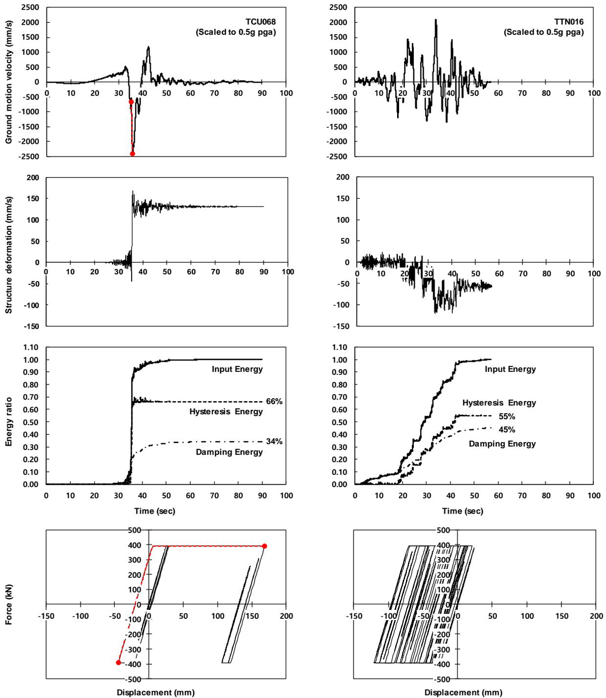
Fig. 3 Inelastic responses of near-fault ground motion, and far-fault ground motion (pga: 0.5g)
