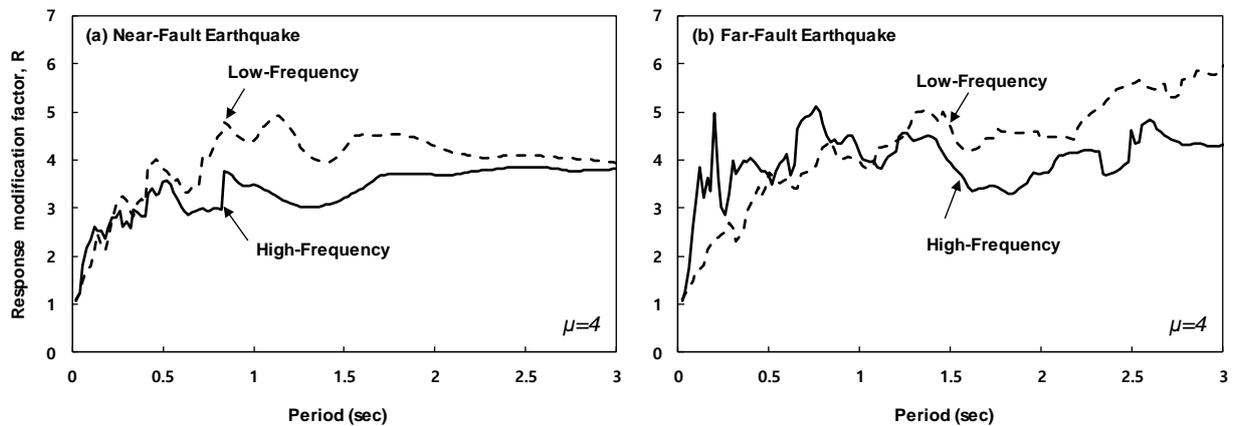
Fig. 6 Response modification factors and earthquake frequency components:
