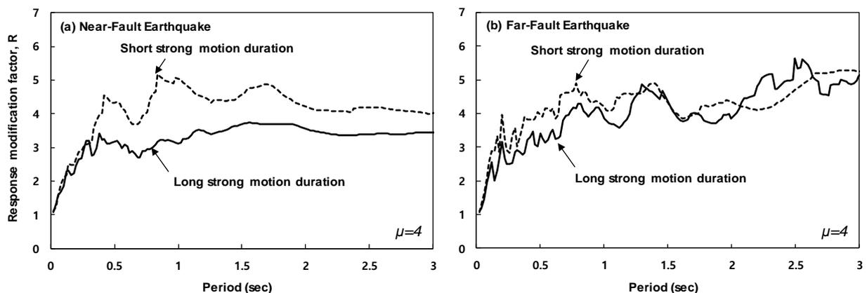
Fig. 7 Response modification factors and strong motion duration:
