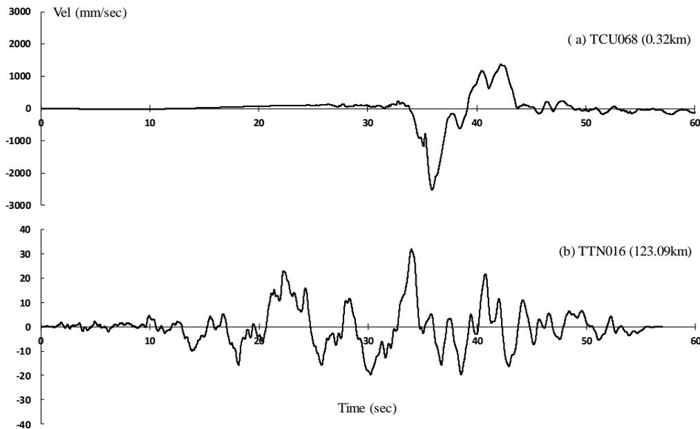
Fig. 2 Chi-Chi earthquake(1999) Ground motion records (a)TCU068 (b)TTN016
