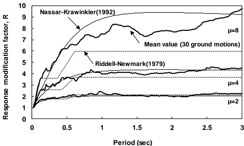
Fig. 4 Average strength reduction factors of 30 ground motions
