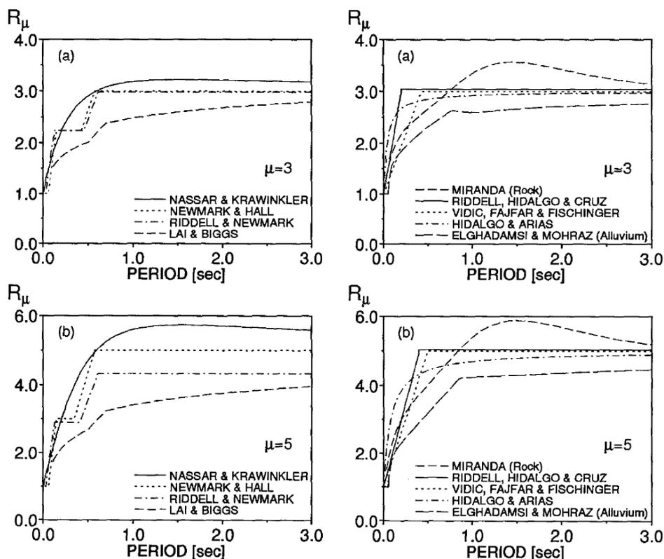
Fig. 1 Comparison of strength reduction factors proposed in various studies for (a) ductility=3, and for (b) ductility=5 (Miranda and Bertero(1994))
