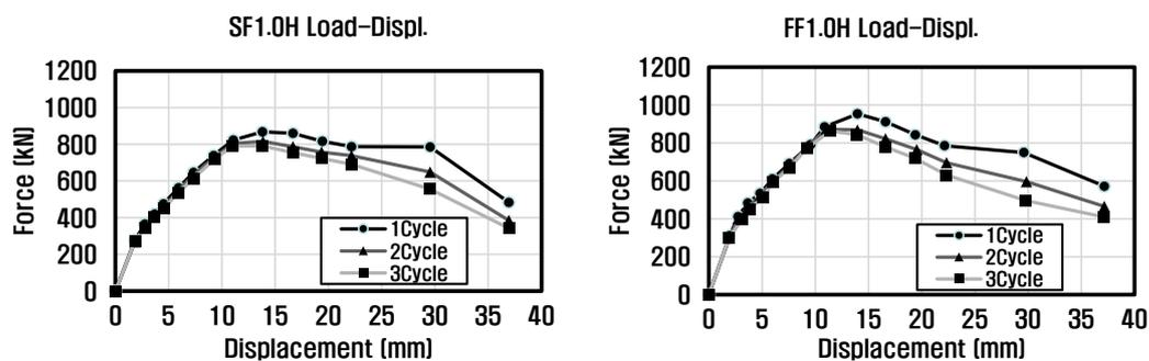
Fig. 1 Flexural Specimen Load-Displacement curve (Left: Static, Right: Dynamic)
