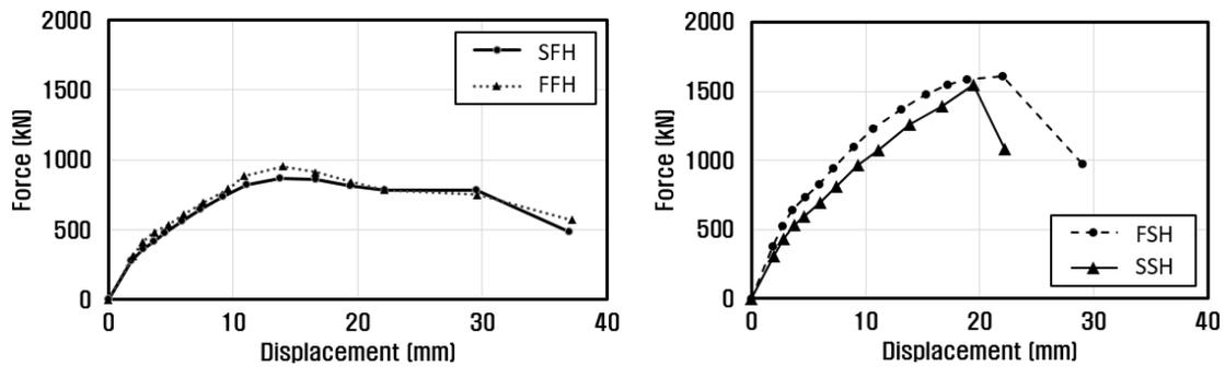
Fig. 2 Envelop of load-displacement (Left: SFH and FFH, Right: SSH and FSH)
