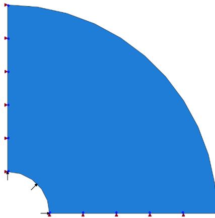
Fig. 4. Finite element model of the pile with constraints and loads
