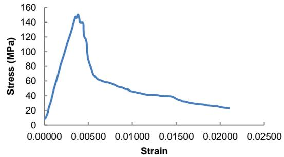
Fig. 3b. Compressive stress-strain graph
