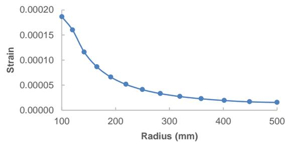
Fig. 6b. circular strain distribution in pile
