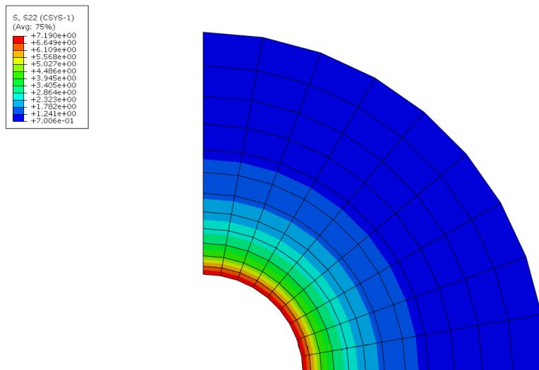
Fig. 5. Circular stress inside the pile section
