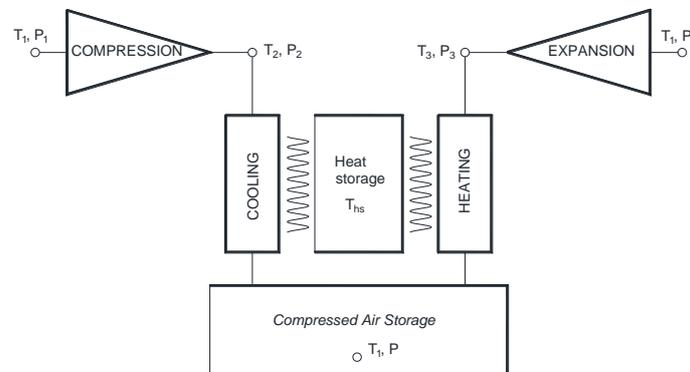
Fig. 1. CAES thermodynamic cycle schematic
