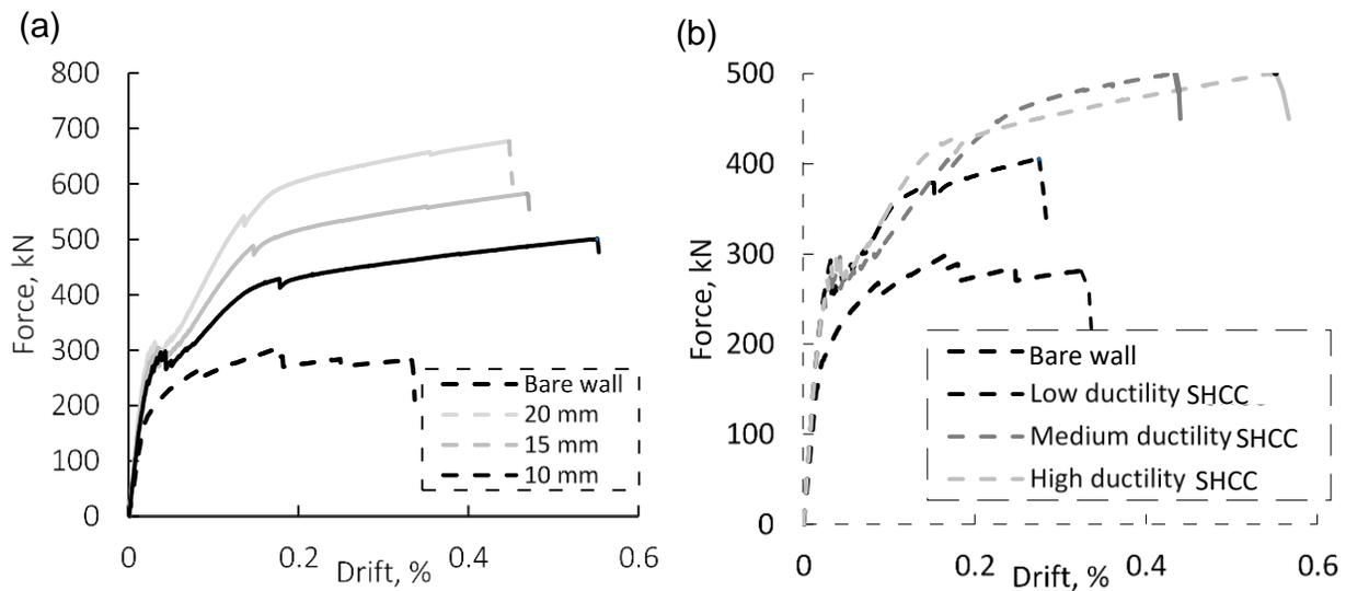
Fig. 2 Pushover curves for different: (a) SHCC thicknesses; (b) SHCC ductility
