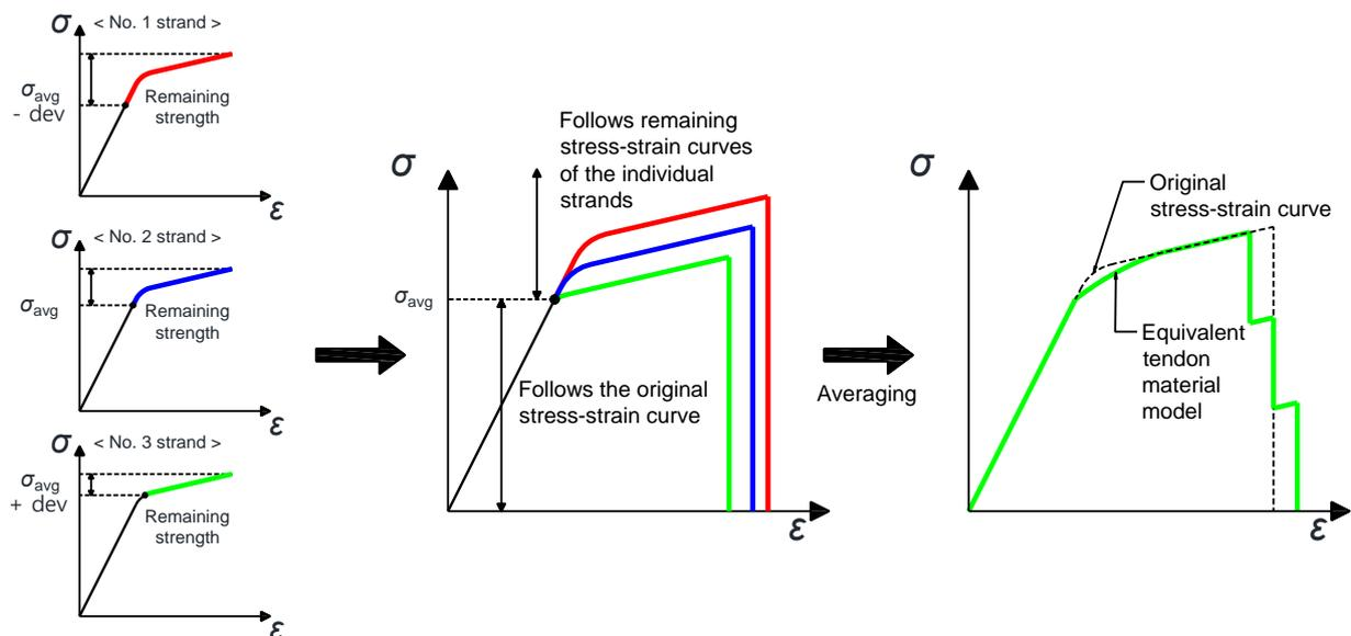
Fig. 1 Concept of equivalent tendon stress-strain relationship
