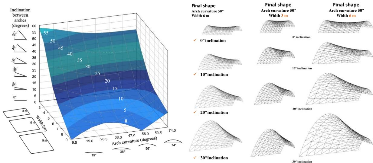
**Fig. 6** Design aid for inclined anticlastic membrane tension structures and final design examples
