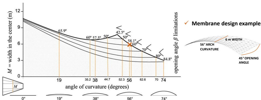
**Fig. 4** Design aid for trapezoid-shaped anticlastic membrane tension structures and final design example
