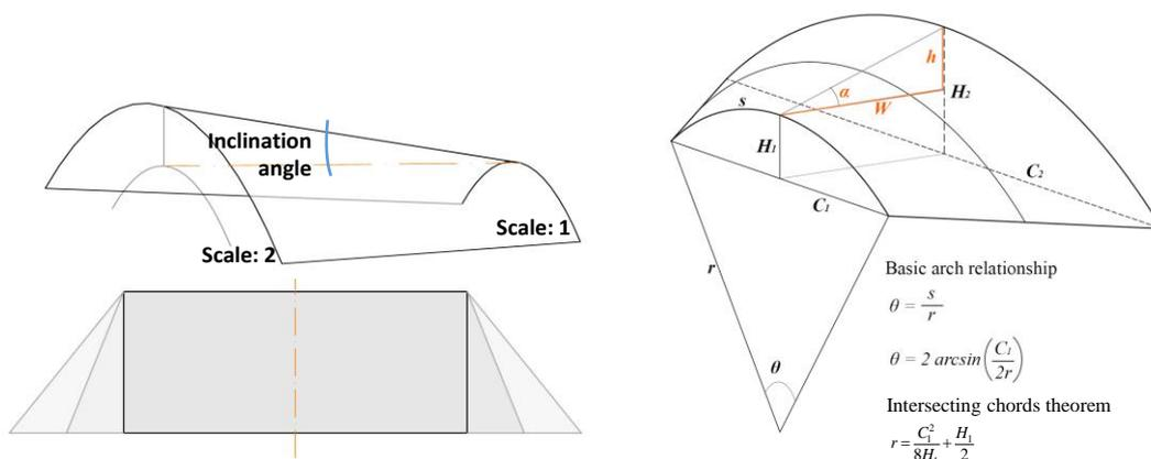
**Fig. 5** Parameters defining scale of larger arch in consideration of inclination angle between two arches
