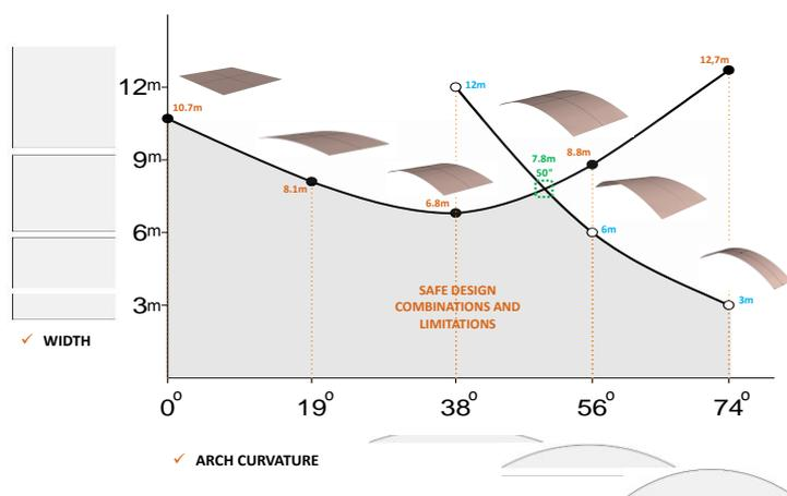
**Fig. 3** Design aid for regular anticlastic membrane tension structures
