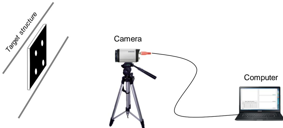
Fig 1. Component of general vision-based displacement measurement
