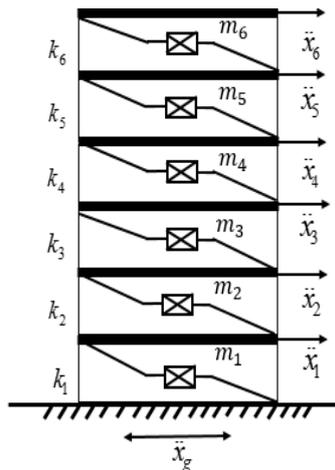
Fig. 1 A 6-floor shear frame building structure
