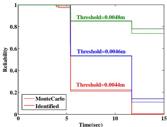
Fig.4 System reliability of undamaged structure
