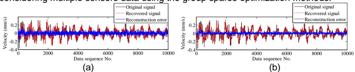
Figure 5. Data reconstruction results from 10% samples: (a) reconstruction from single sensor data; (b) reconstruction from group sensors data
