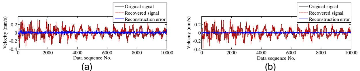
Figure 6. Data reconstruction results from 30% samples: (a) reconstruction from single sensor data; (b) reconstruction from group sensors data sets
