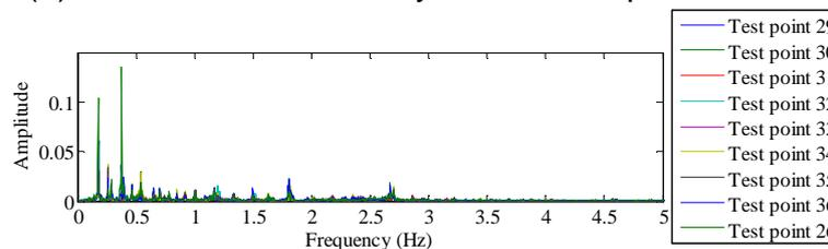
(b) The Fourier spectrum of the measured velocity data of test points 29-36
