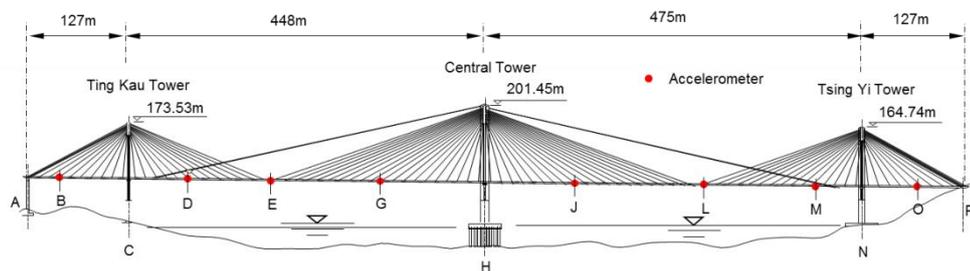
Figure 1 Layout of accelerometers on bridge deck
