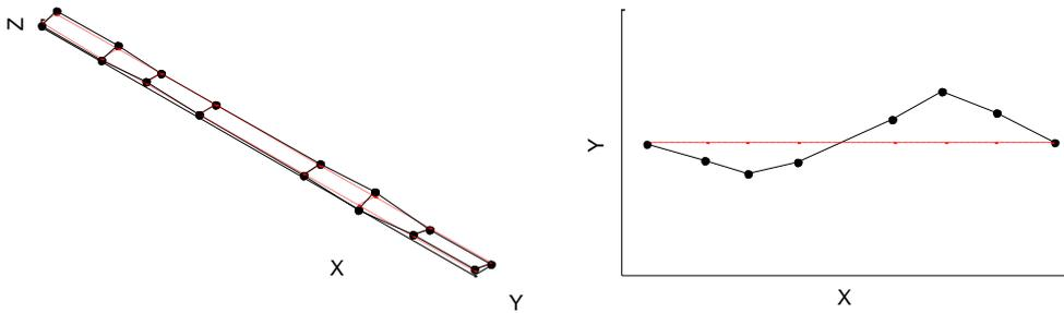
Figure 4 Mode shape of the 3rd mode from Sample 1
