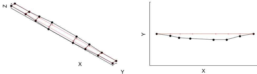
Figure 6 Mode shape of the 2nd mode from Typhoon York 1 (0.227 Hz, 0.40%)
