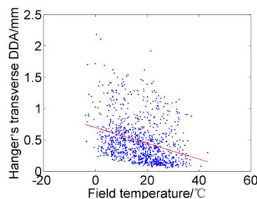
Fig. 4 Relationship between temperature and the train-induced hanger's transverse DDA for train load case 1
