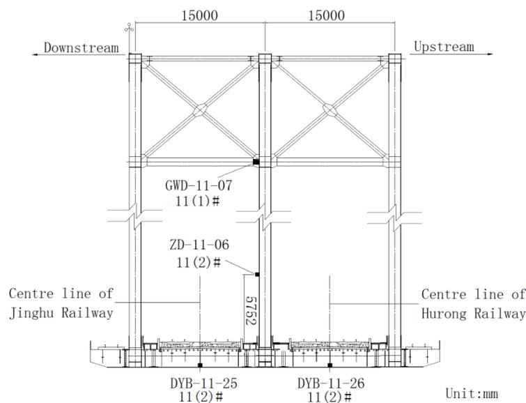
Fig. 2 Sensor Layout Diagram in 11# Section
