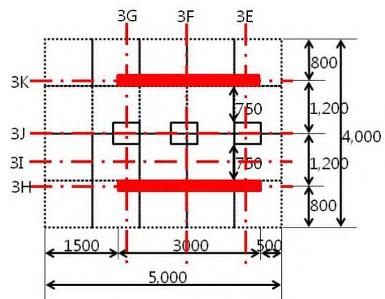
Fig. 2 GPR detection lay out (unit:mm)
