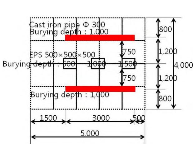
Fig. 1 Test bed plan (unit:mm)
