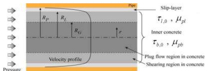
Figure 1: Profile of flow of concrete in a pipe [2]
