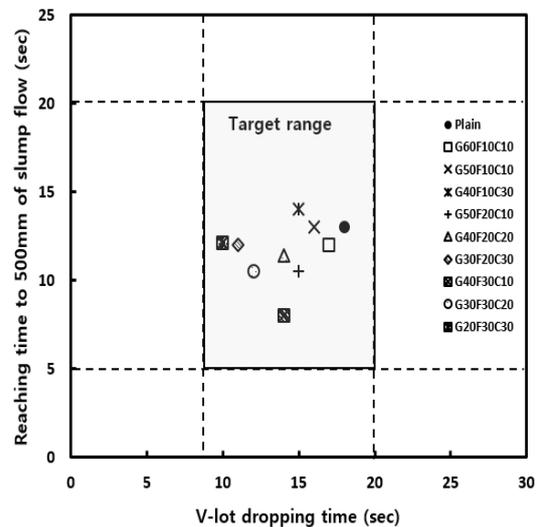
Fig. 6. Reaching time to 500 mm of slump flow
