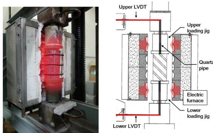
Fig. 2 Experimental apparatus used in this study
