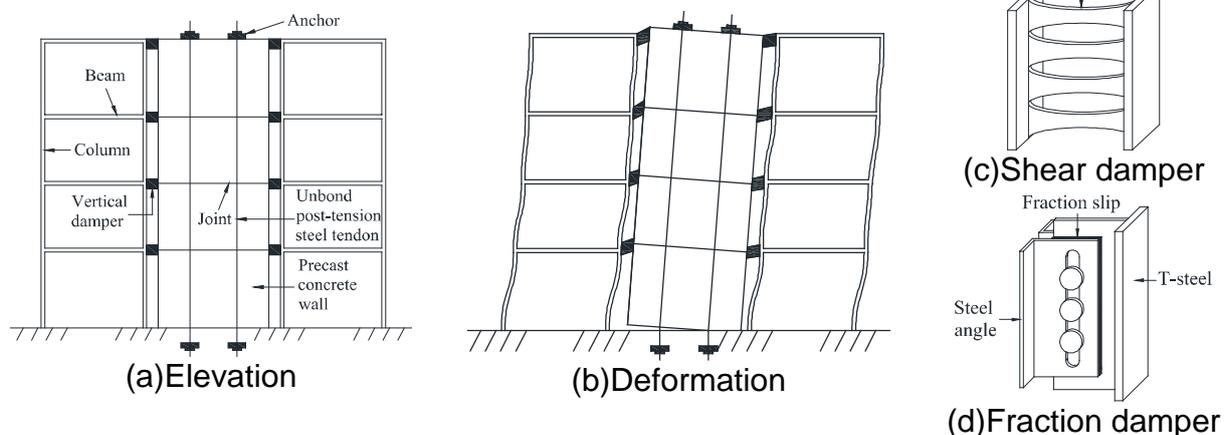
Fig. 1 The concept of frame-SCW system with Vertical dampers
