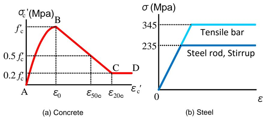
Fig. 7 Stress-strain curves
