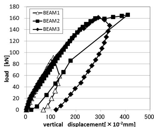
Fig. 3 Load-deflection curve (BEAM1, BEAM2 and BEAM3)
