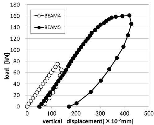
Fig. 4 Load-deflection curve (BEAM4 and BEAM5)
