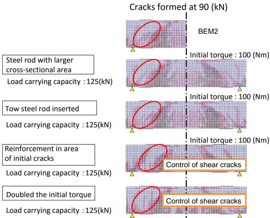
Fig. 9 Analysis results with different reinforcement conditions
