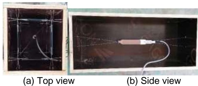
Fig. 3 Installation of embedded strain gauge
