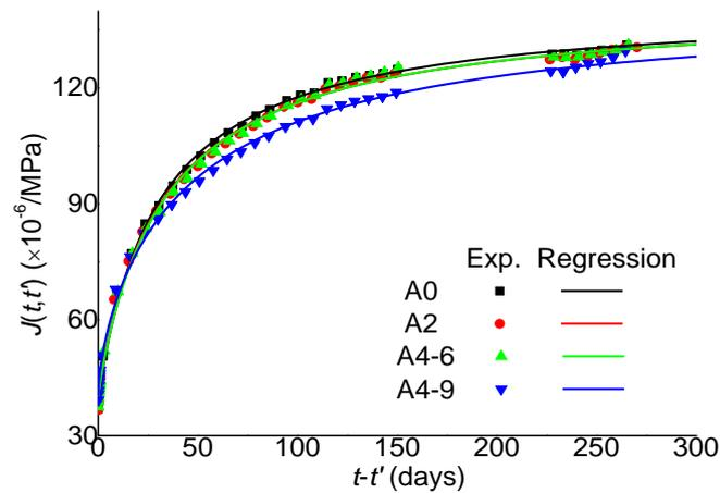
Fig. 6 Creep compliances of columns and regression results
