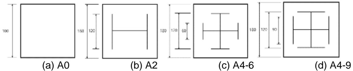
Fig. 2 Cross-sectional plan of columns
